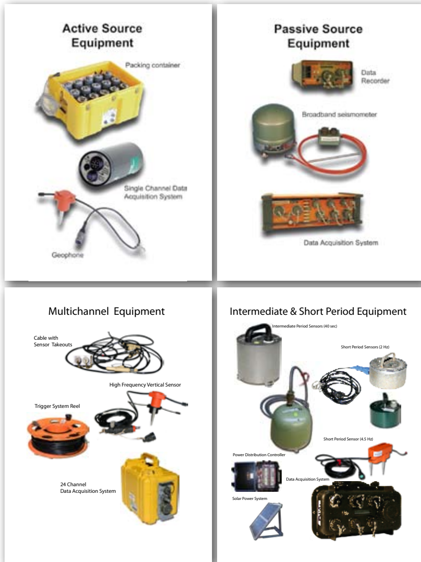
Figure A2.5. PASSCAL major equipment. Instrumentation provided and supported by the PASSCAL facility can be divided into four categories: active source, passive source broadband, intermediate and short period, and multichannel.
