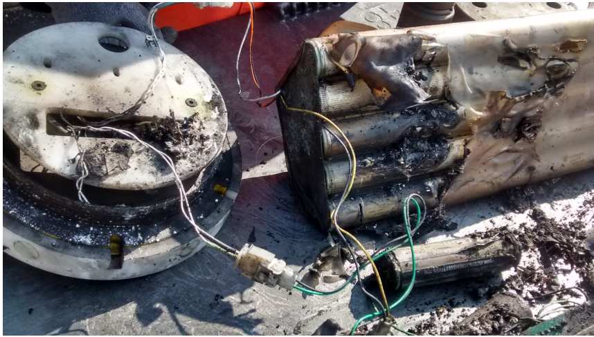
Remnants of a battery pack after undergoing combustion
