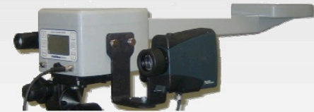
As seen with options: Laser Technology Inc. TruPulse Laser and Alignment Scope
