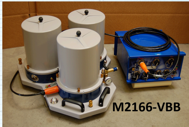
Prototype vault sensor being tested
