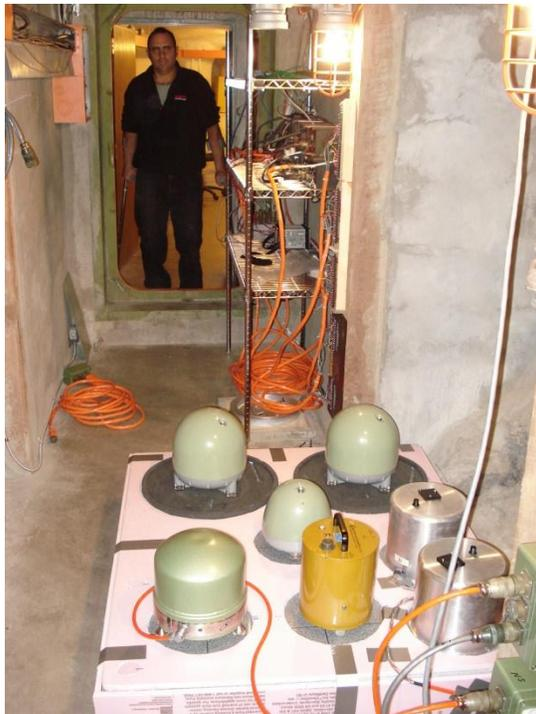
Figure 5c: View from center of cross tunnel toward west ship door, showing Leo Sandoval preparing to perform a “huddle test” of several instruments on the granite slab.
