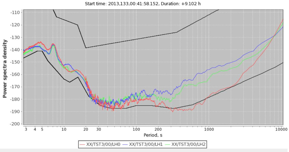
Figure 6: Typical long-period noise levels from STS-1 reference seismometers in cross tunnel during quiet conditions (little or no wind). Red = Z, Blue = NS, Green = EW. Upper and lower black lines are Peterson's (1993) New High Noise Model (NHNM) and New Low Noise Model (NLNM), respectively.
