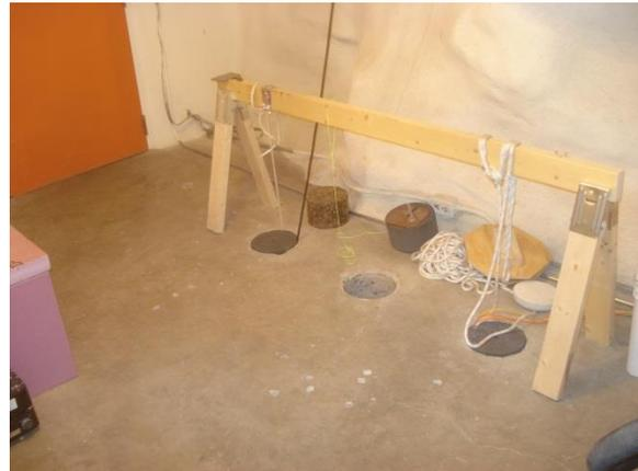
Figure 5h: Three 8'' diameter, 12' deep uncased holes in floor of West Vault used for testing posthole and borehole sensors.
