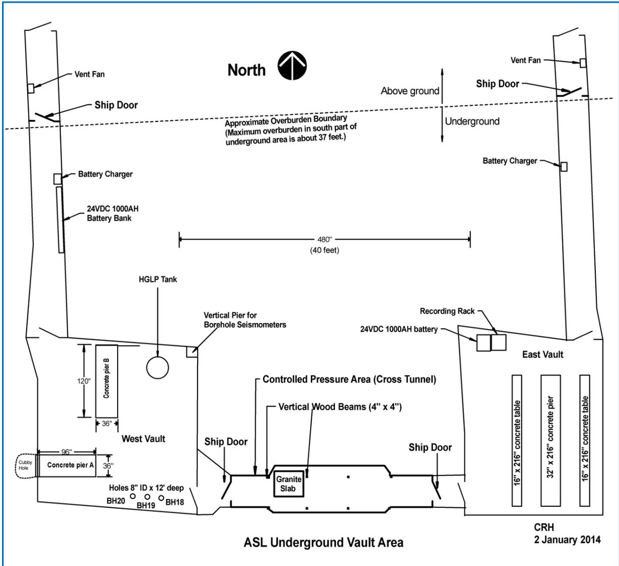
**Figure 4: Underground vault test area. The “Controlled Pressure Area,” also known as the Cross Tunnel, has reduced atmospheric pressure variations at periods shorter than about 20 seconds and very low temperature variations when the ship doors at both ends are closed. The shallow boreholes indicated as BH18, BH19, and BH20 are described in Table 1. 24VDC battery power is available with capacity sufficient to operate sensors and data loggers for several days with AC power turned off.**
