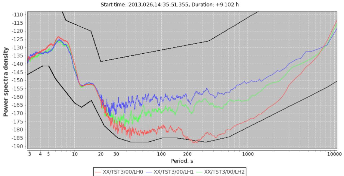
Figure 7: Typical long-period noise levels from STS-1 reference seismometers in cross tunnel during noisy conditions (wind blowing). Red = Z, Blue = NS, Green = EW. Upper and lower black lines are NHNM and NLNM, respectively. The long-period noise level in the N-S direction (blue) is nearly always higher than in the E-W direction, most likely due to the geometry and orientation of the cross tunnel.
