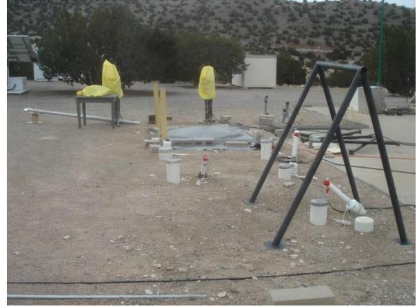
Figure 11b: Five shallow PVC-cased boreholes that terminate in the soil layer. Two steel-cased boreholes are in the background (with yellow bags over them).
