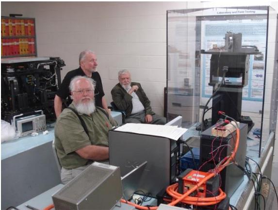
**Figure 15c:** John Evans, with Czech Academy of Science colleagues, using the Aerotech rotational shaking table to test rotational sensors.
