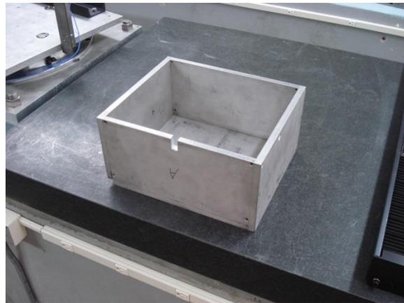
**Figure 15d:** Box having faces that are precisely orthogonal, sitting on the dead-level granite precision surface plate. This surface is level to within 0.001" per foot. Used for determination of accelerometer sensitivity and axis orientation.
