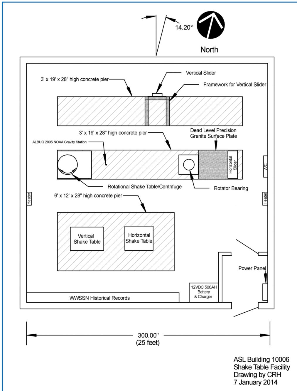
**Figure 14: Shake Table Facility.** This is a 25' x 25' surface building with large concrete piers poured directly on outcropping Pre-Cambrian granite. It contains several shaking tables and other devices used for both static and dynamic testing various types of ground motion sensors. 12 VDC battery power is available.
