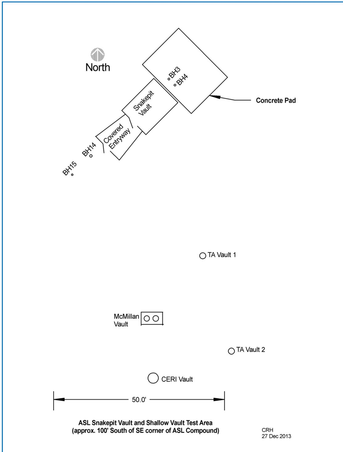
**Figure 12: Shallow vault test area. The “Snakepit Vault” is a partially buried concrete block building with the roof exposed at ground level. The concrete floor is in direct contact with granite. See Table 1 for a brief description of boreholes BH3, BH4, BH14, and BH15. The other shallow vaults are described in the text. Scale is approximate.**
