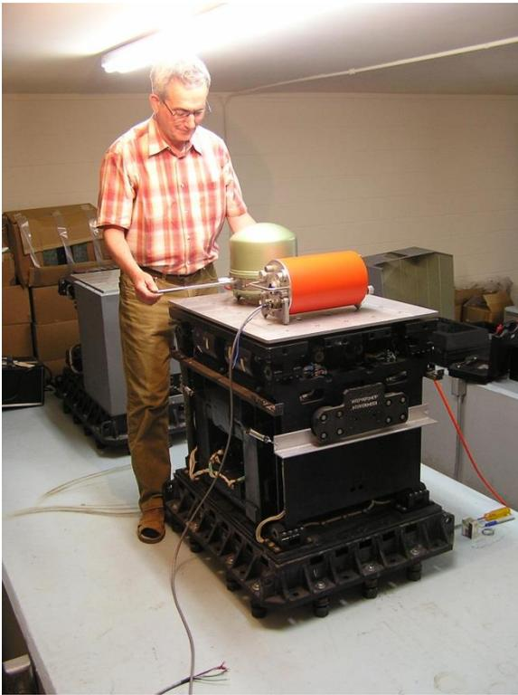
**Figure 15a:** Erhard Wielandt using horizontal shaking table to determine cross-axis sensitivity of an STS-2 BB seismometer. Vertical table is in background.
