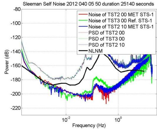
Figure 5f: Example of determination of self-noise of two vertical VBB instruments under test (00 MET STS-1 and 10 MET STS-1) by comparison with the reference STS-1V buried under sand. The ship doors on both ends of the cross tunnel must remain closed for extended periods (several days) in order to achieve good test results in the low frequency band (0.001 Hz to 0.05 Hz ).
