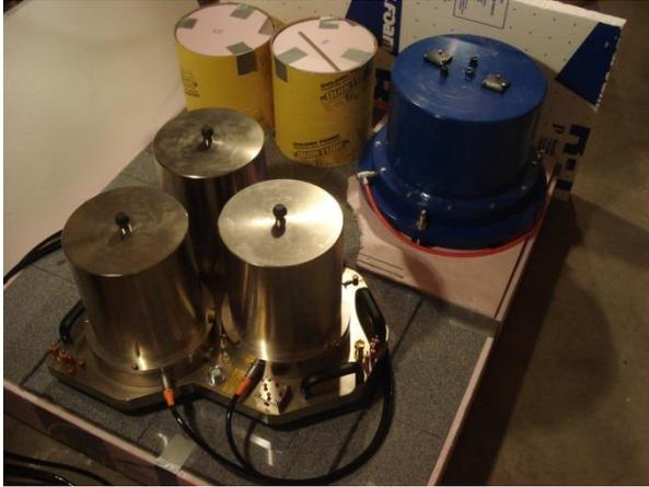
Figure 5e: Seismometers under test on granite slab in Cross Tunnel. The slab is supported by three lead pads for coherent tilt across the entire surface, allowing better determination of horizontal instrument self-noise in the long period band. When noise test data are being collected, the slab and instruments are shielded against stray air currents and thermal fluctuations with a 2-inch thick insulating foam box.
