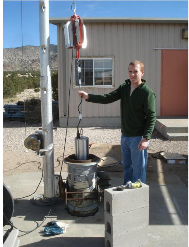
Figure 11d: Adam Ringler preparing to lower a Trillium T120PH seismometer into 106.7m deep, 12 5/8" diameter hole for noise testing. This large diameter borehole is also known as the "Russian Borehole," as it was drilled for testing a Russian BB seismometer in 1990. This seismometer had a diameter of 9 inches, too large to fit into the standard 6.5" ID boreholes.
