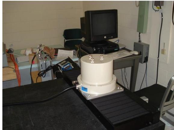
**Figure 15b:** Using Anorad horizontal positioning stage ("horizontal slider" in Figure 10) to perform velocity-to-displacement integration test of a strong motion velocity sensor. The horizontal positioning stage is mounted on the dead-level granite precision surface plate that is also used for "box flip tests" of accelerometers.
