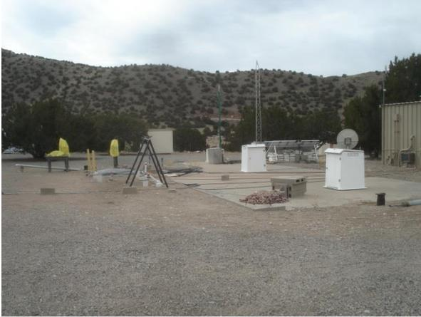
Figure 11a: Main ASL borehole test area. ANMO boreholes are under the two white covers.
