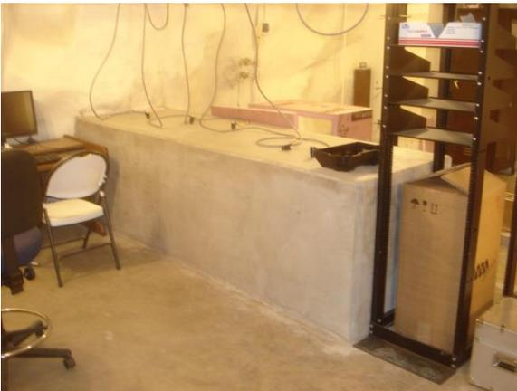
Figure 5g: Pier in West Vault typically used for testing strong motion sensors (accelerometers).
