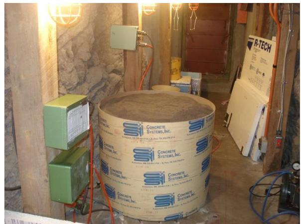
Figure 5d: View looking east into cross tunnel. STS-1V/VBB seismometer is in evacuated chamber under a large amount of sand for excellent temperature stability.
