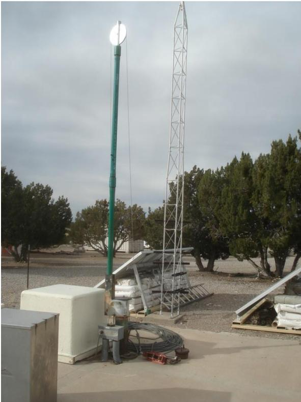
Figure 11c: Deep (150m) steel-cased hole used for testing KS54000 and other BB and VBB borehole seismometers. Mast with pulley on top is used to support seismometer over hole when installing and retrieving the instrument.
