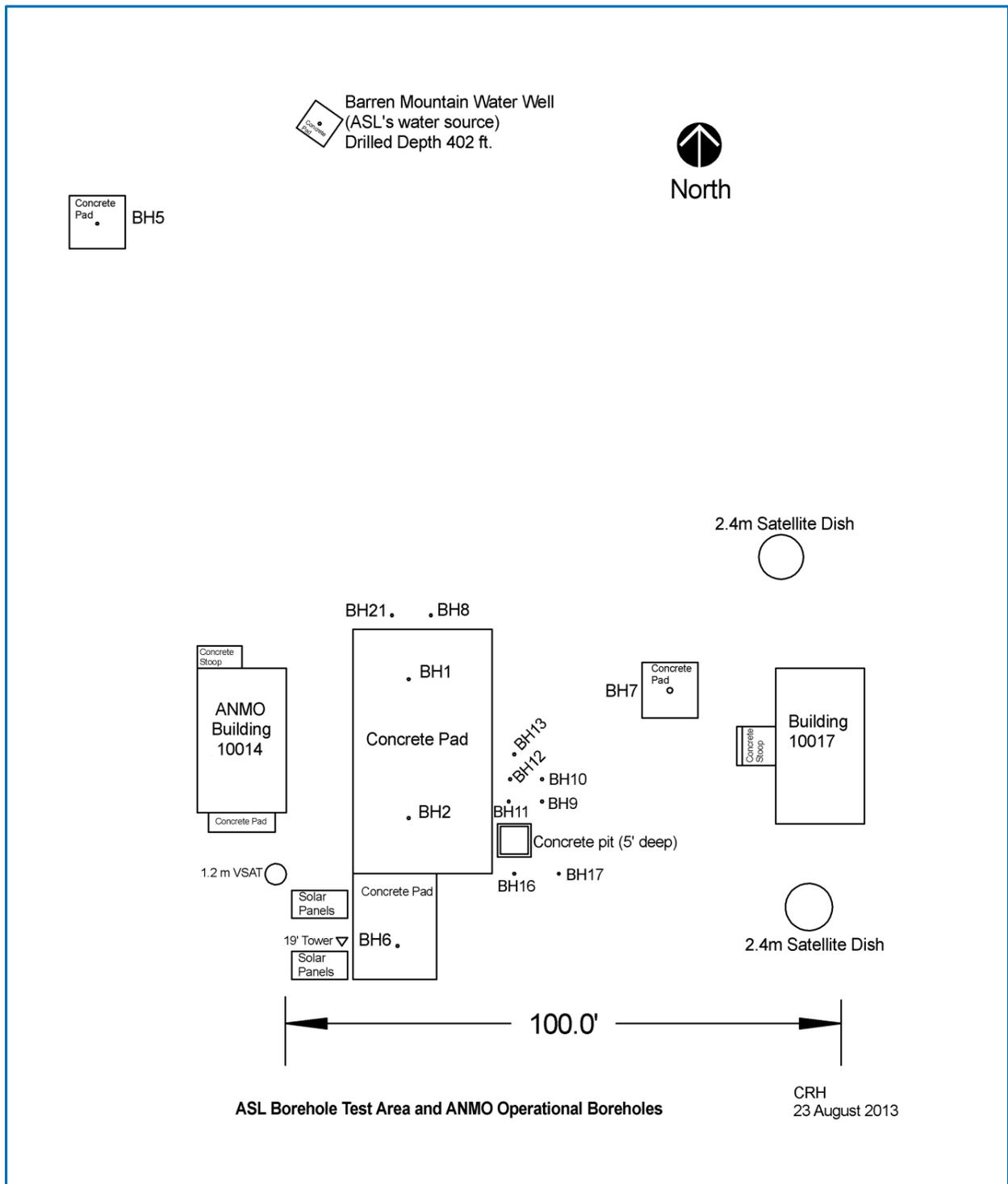
**Figure 10: Main borehole test facility. Scale is approximate. Depths and diameters of boreholes are listed in Table 1. Boreholes 10 and 11 (BH10 and BH11) contain the two ANMO broadband borehole seismometers.**
