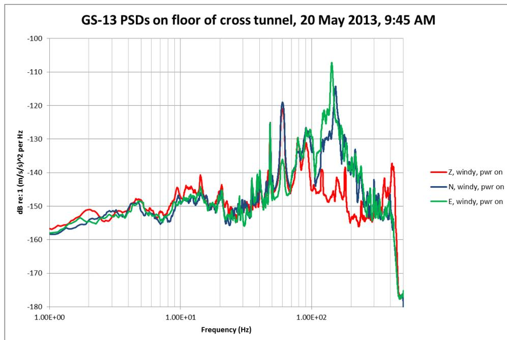
Figure 9: Typical high-frequency noise levels from Geotech GS-13 seismometers in cross tunnel during noise conditions (windy, vault power on, ventilation fans on, daylight hours), window length 66 seconds. Red = Z, Blue = NS, Green = EW. Peterson's (1993) NLNM is at -168 dB from 1 Hz to 10 Hz. A level of -160 dB on this plot roughly corresponds to 1 nano-g per root Hz. Peaks above 100 Hz in horizontal components are instrumental in origin (internal resonances in the GS-13 seismometers).
