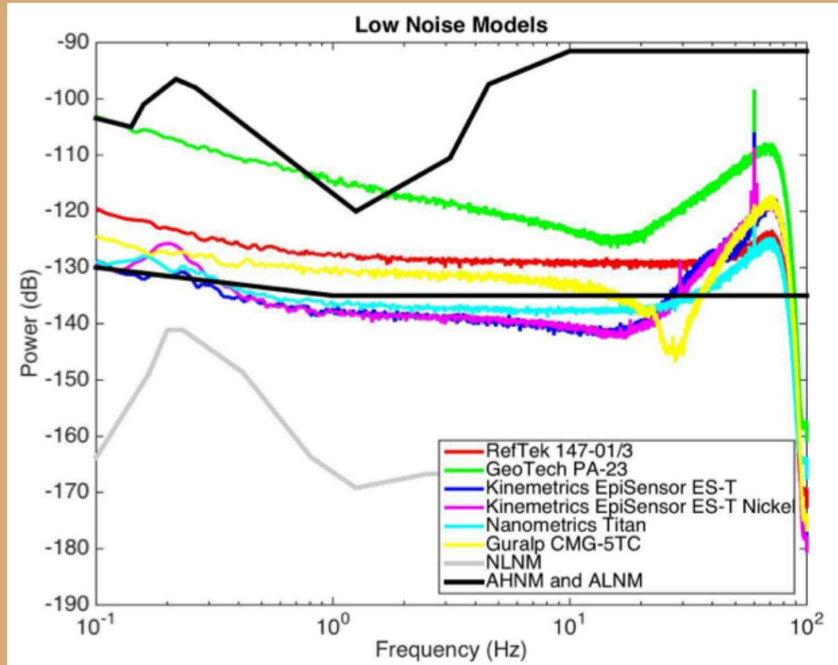
Not using coherence since site noise is below sensor noise
