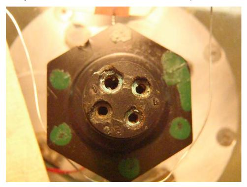
• Transducer corrosion
