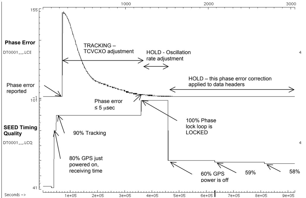
Figure 1. Q330 timing as illustrated by the Baler LCE (phase error) and LCQ (timing quality) channels.
