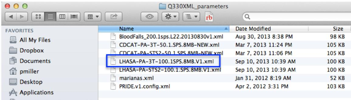
Select Configuration -> Configuration Cloning and select Load from File. Browse to the XML configuration file to be used, select it and click Open.
