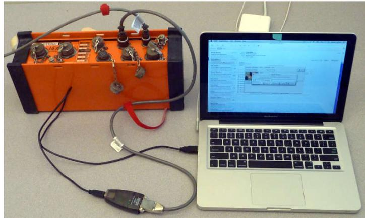
With the powered Q330 connected to a computer via the serial/USB ports, open the Willard application. It will come up with a prompt for a station. Select the Console Registration button.
