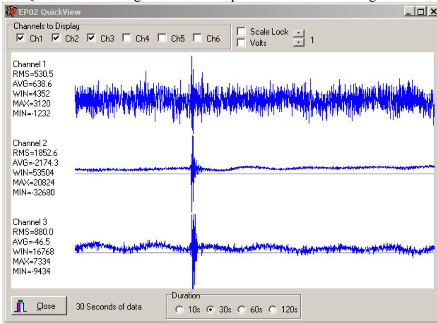
The plot is auto-scaling and with a sensor connected, the signal from a stomp test will be visible as a simple operational test of the sensor and Q330.
