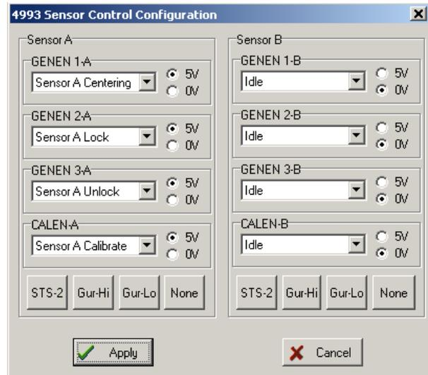
These settings should be adjusted and applied BEFORE connecting a sensor. Also, the sensor configuration should be saved to the EEPROM so that if the Q330 loses power it will reboot with the correct configuration. From the Command menu select System and GPS control, then check the Reboot Q330 and Save to EEPROM boxes and click Apply.
