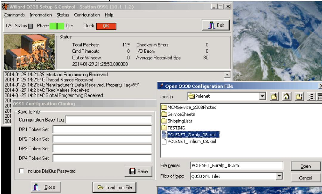
After the file has finished loading, all of the fields in the Configuration Load window will be empty. Select Copy from File for DPs, Interface and Global. This will copy the specified names and values from the file. The station names should now indicate the generic configuration. Select Apply.
