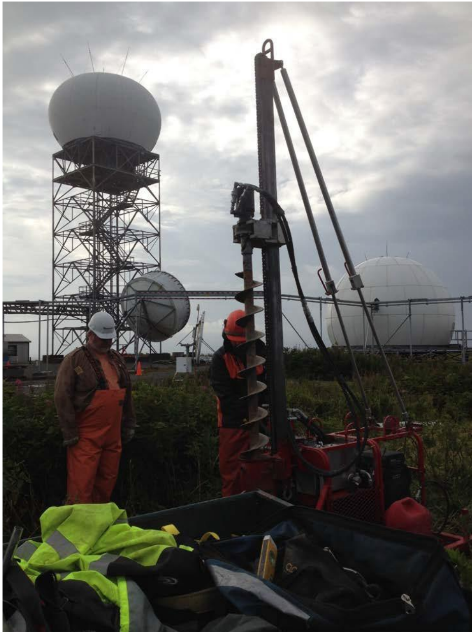
Figure 2: Red Drill onsite in auger drilling mode
