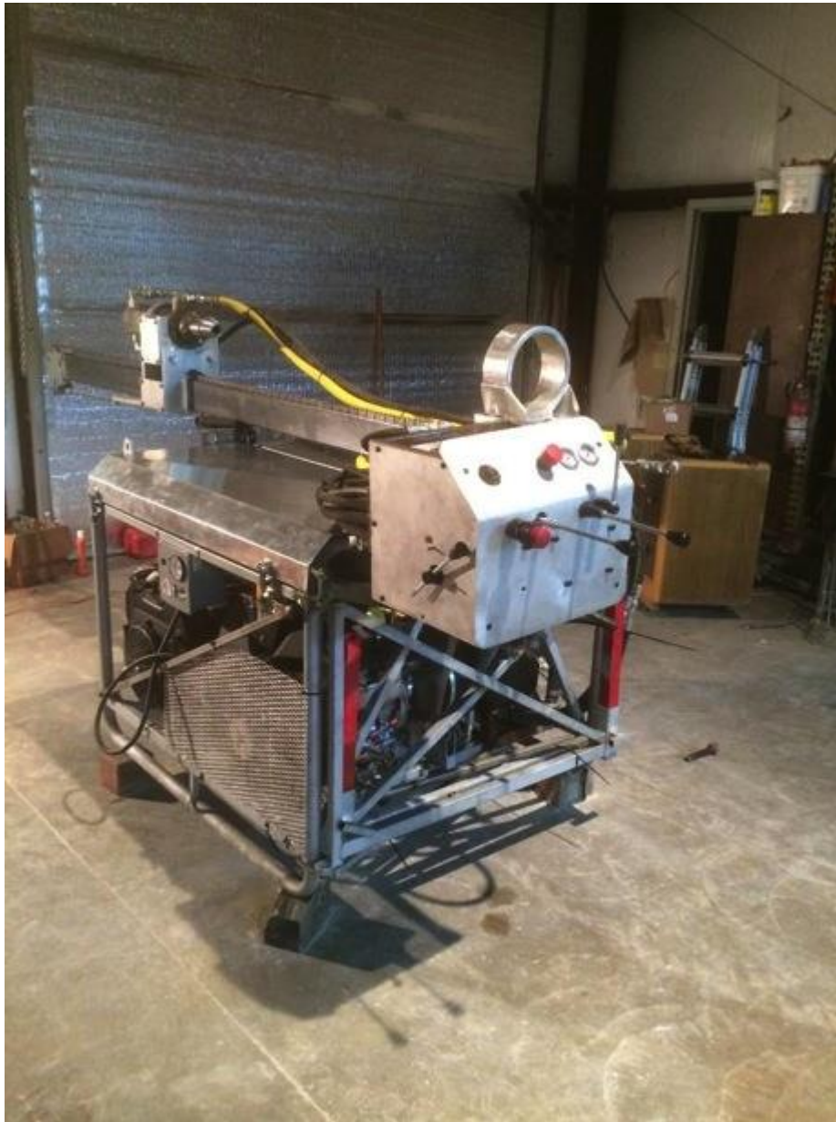
Figure 4: Silver Drill in transit configuration
