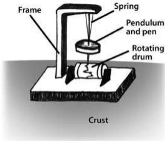
24. What keeps the stable part of this seismometer from moving during an earthquake?
