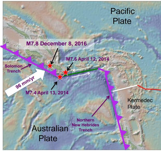
This earthquake occurred along a portion of the Australian–Pacific Plate boundary. The Australian Plate subducts beneath the Pacific Plate at the Solomon and Northern New Hebrides trenches. Along with its location and depth, the thrust faulting mechanism of the M7.8 December 8, 2016 earthquake indicates that it occurred on the Solomon Trench subduction zone boundary.
