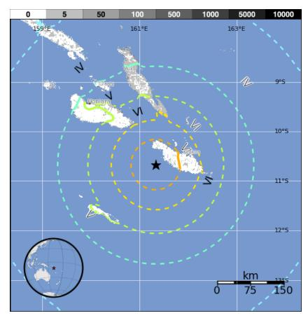
The color coded contour lines outline regions of MMI intensity. The total population exposure to a given MMI value is obtained by summing the population between the contour lines. The estimated population exposure to each MMI Intensity is shown in the table.
