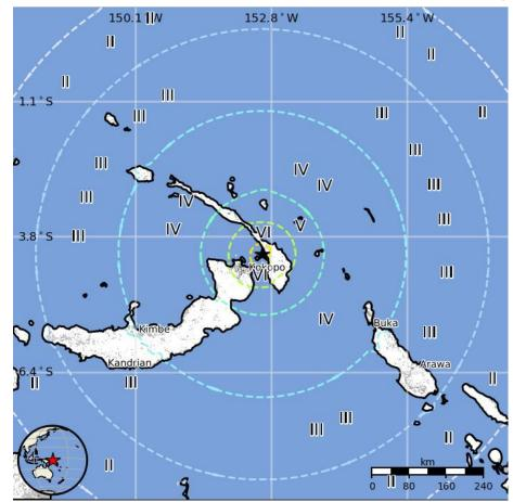
The color coded contour lines outline regions of MMI intensity. The total population exposure to a given MMI value is obtained by summing the population between the contour lines. The estimated population exposure to each MMI Intensity is shown in the table.
