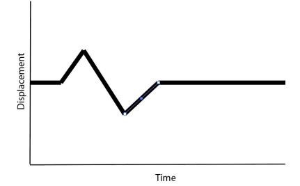
**Example 2:** The ground at the seismometer... <u>moved up a little, then down past the original</u> <u>position a little, and then back to the original position.</u>
