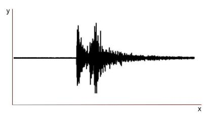
• On the seismogram above from last week, label the x-axis time and the y-axis ground displacement.
