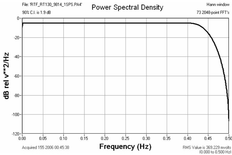
Figure 6.10.5c Response of the RT130HR to Broadband Noise
