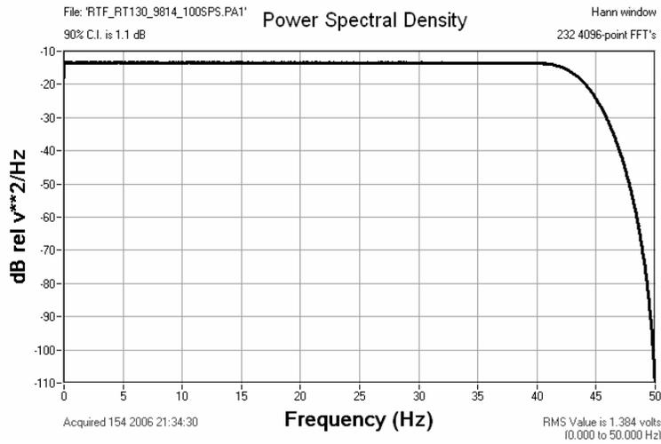
Figure 6.10.2a Response of the RT130HR to Broadband Noise
