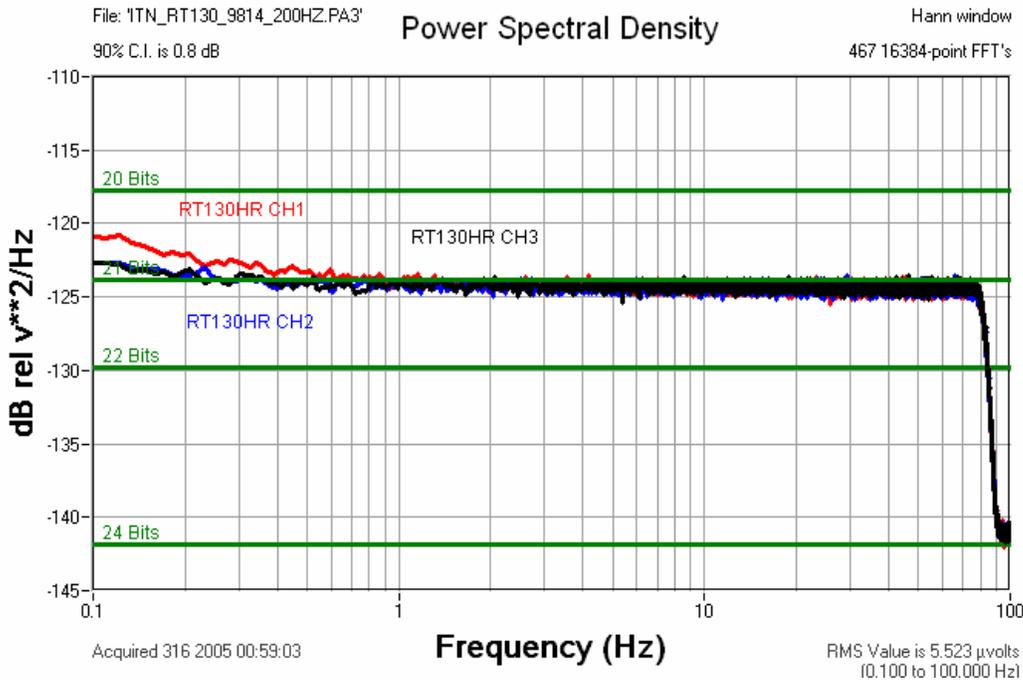
Figure 6.7.1 RT130HR 200SPS Channel 1-3 Input Terminated Noise
