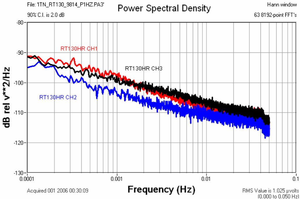
Figure 6.7.9 RT130HR 0.1SPS Channel 1-3 Input Terminated Noise
