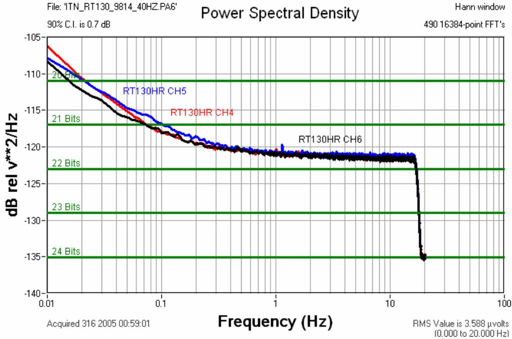
Figure 6.7.5 RT130HR 40SPS Channel 4-6 Input Terminated Noise
