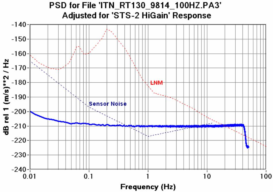
Figure 6.12.2c RT130HR 100SPS CH3 Seismic System Noise STS-2 High Gain
