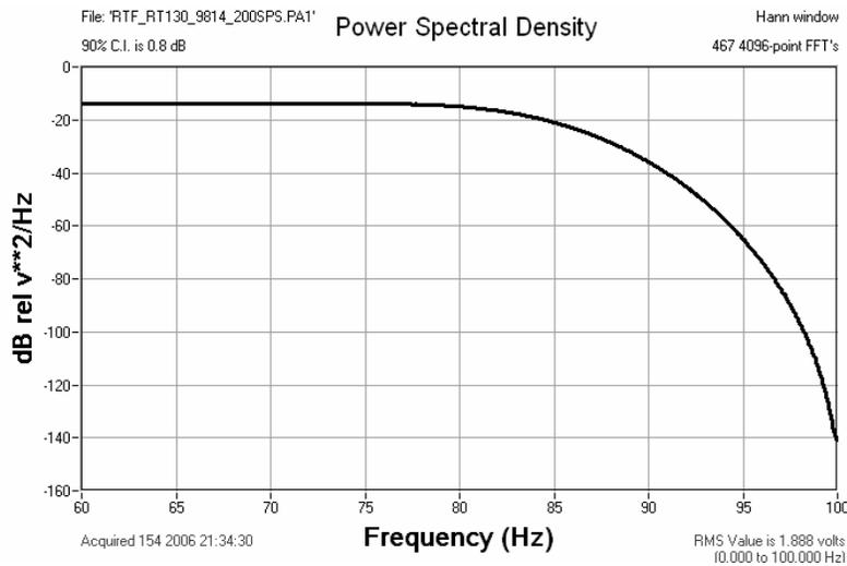
Figure 6.10.1b Response of the RT130HR to Broadband Noise
