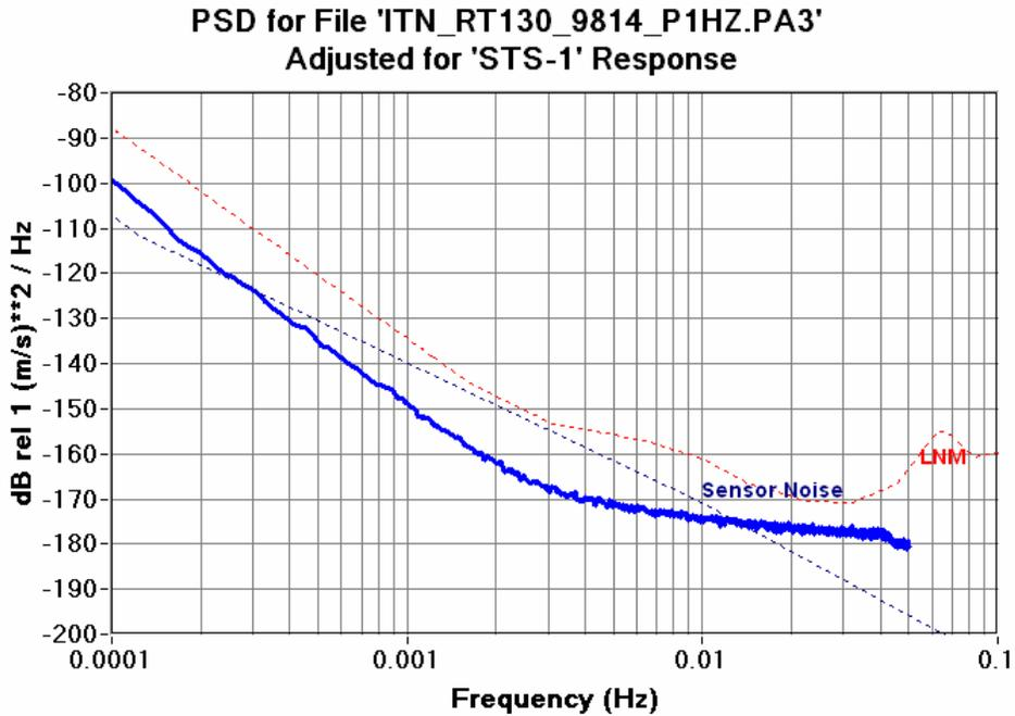
Figure 6.12.16c RT130HR 0.1SPS CH3 Seismic System Noise STS-1
