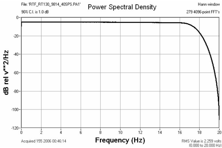
Figure 6.10.3c Response of the RT130HR to Broadband Noise
