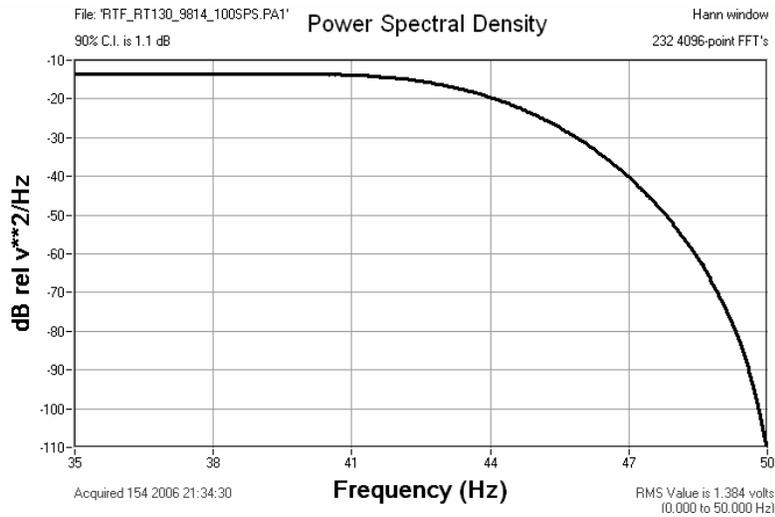
Figure 6.10.2b Response of the RT130HR to Broadband Noise
