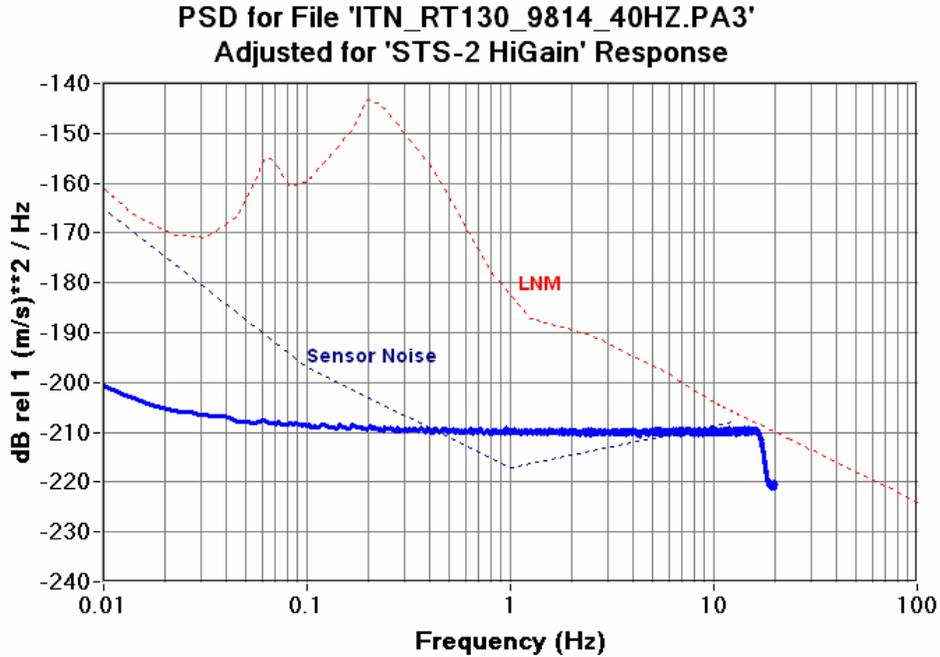
Figure 6.12.4c RT130HR 40SPS CH3 Seismic System Noise STS-2 High Gain
