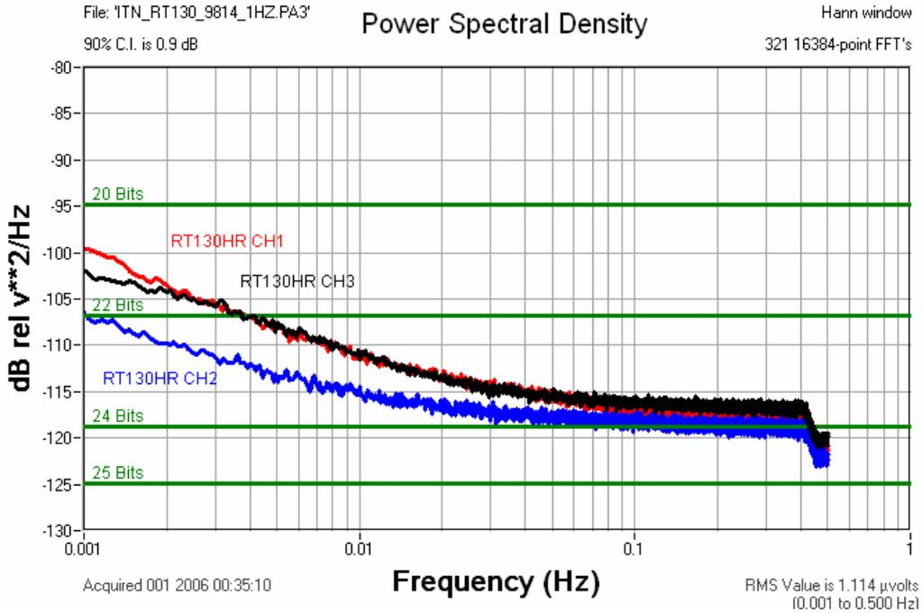
Figure 6.7.7 RT130HR 1SPS Channel 1-3 Input Terminated Noise
