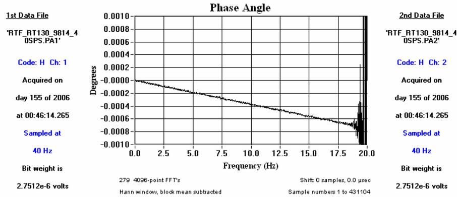
Figure 6.10.3a RT130HR 40SPS Channel 1-2 Relative Phase/Skew
