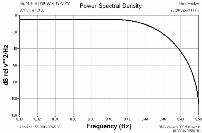
Figure 6.10.5b Response of the RT130HR to Broadband Noise
