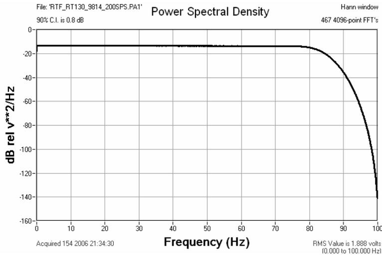
Figure 6.10.1a Response of the RT130HR to Broadband Noise
