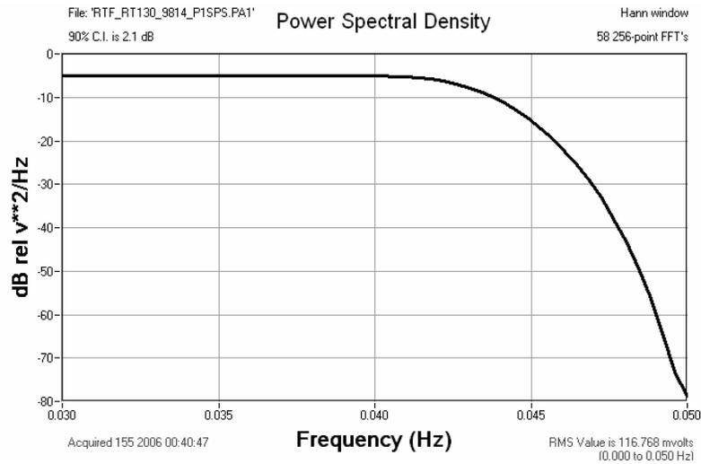
Figure 6.10.6b Response of the RT130HR to Broadband Noise
