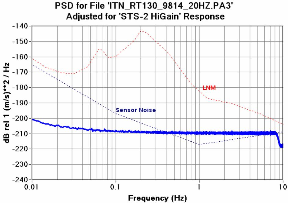
Figure 6.12.7c RT130HR 20SPS CH3 Seismic System Noise STS-2 High Gain
