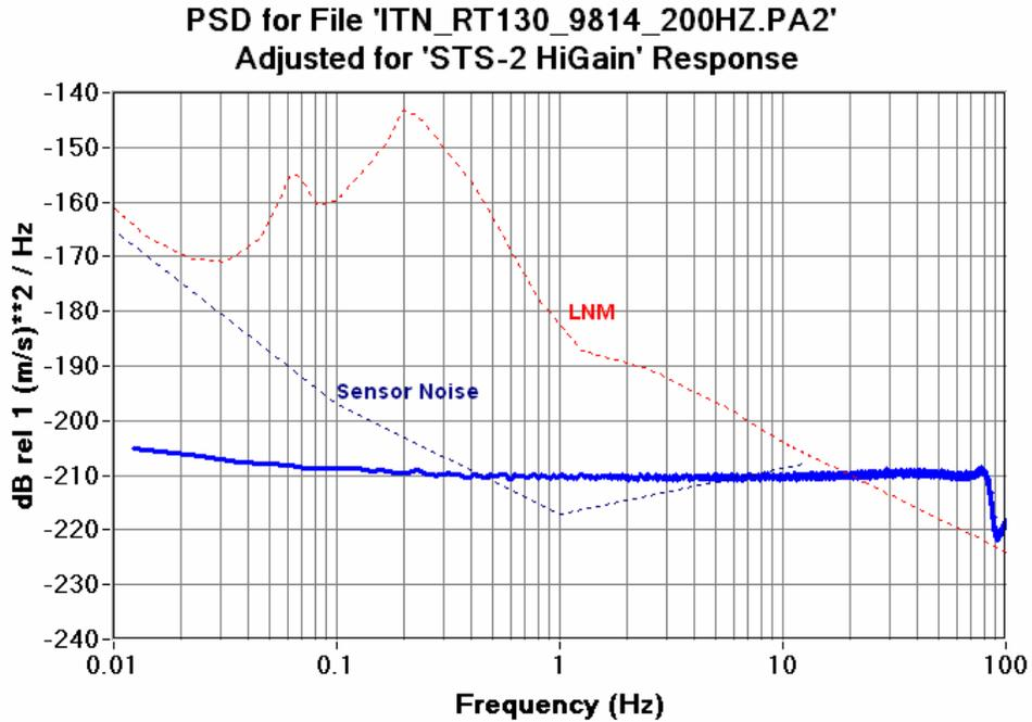
Figure 6.12.1b RT130HR 200SPS CH2 Seismic System Noise STS-2 High Gain
