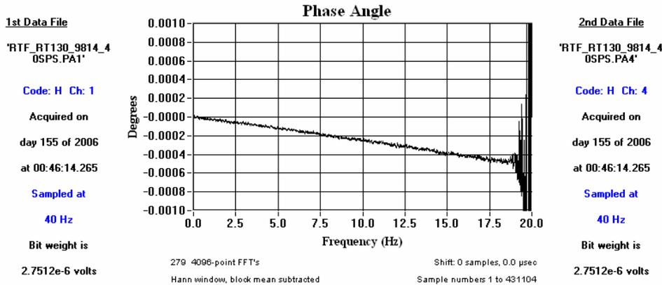
Figure 6.10.3b RT130HR 40SPS Channel 1-4 Relative Phase/Skew
