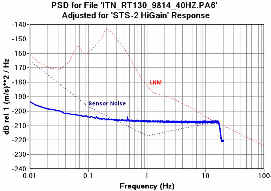
Figure 6.12.6c RT130HR 40SPS CH6 Seismic System Noise STS-2 High Gain
