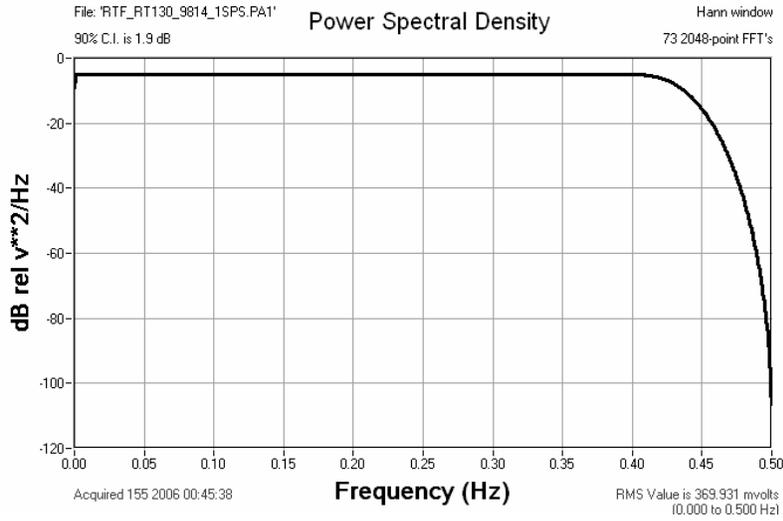
Figure 6.10.5a Response of the RT130HR to Broadband Noise
