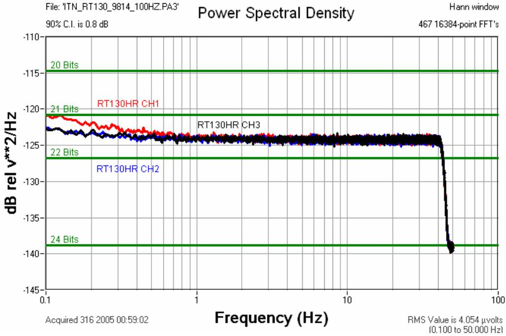
Figure 6.7.2 RT130HR 100SPS Channel 1-3 Input Terminated Noise
