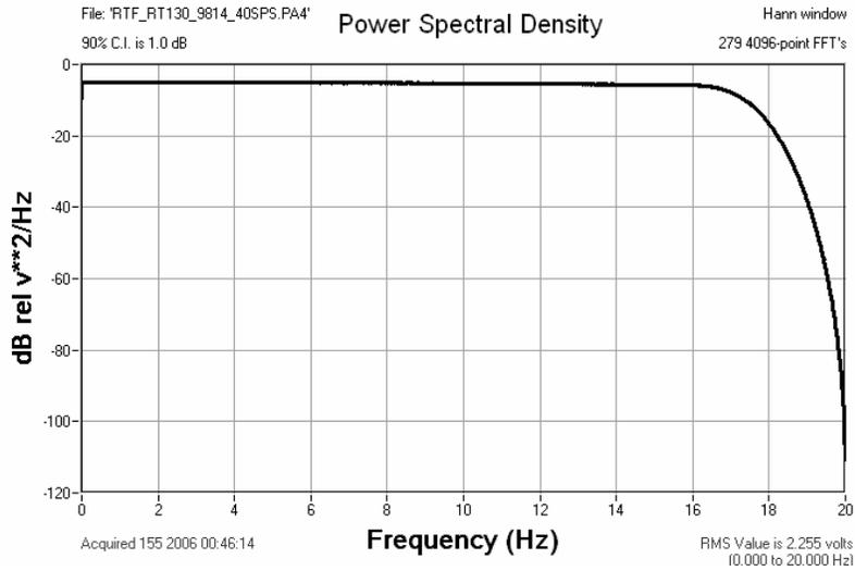
Figure 6.10.3e Response of the RT130HR to Broadband Noise
