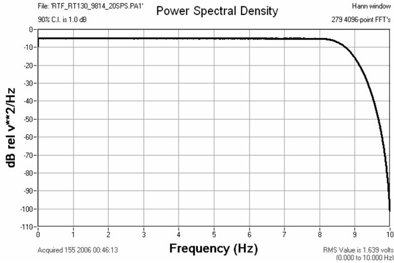
Figure 6.10.4a Response of the RT130HR to Broadband Noise
