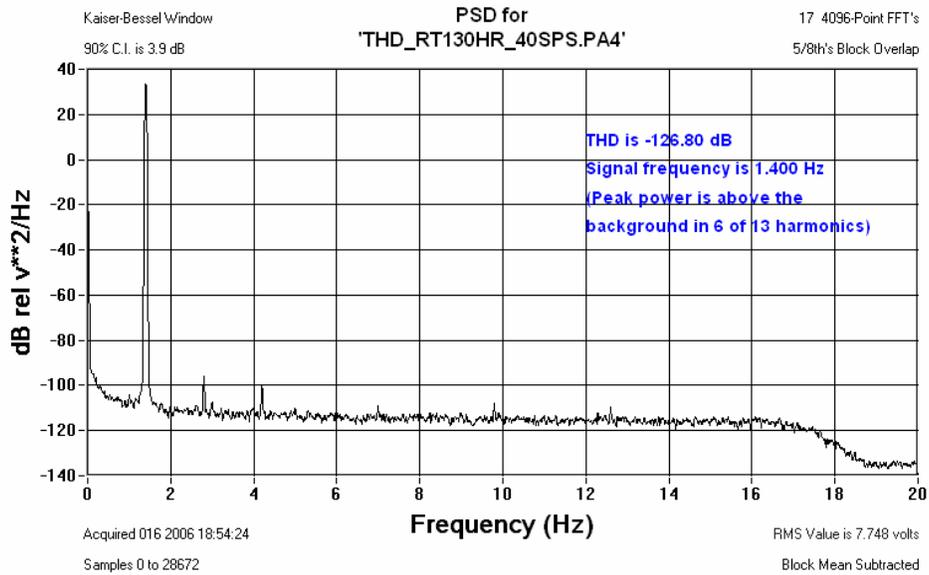
Figure 6.8.2 RT130HR Channel 4 Total Harmonic Distortion
