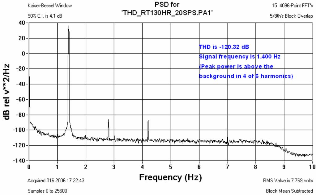
Figure 6.8.3 RT130HR Channel 1 Total Harmonic Distortion
