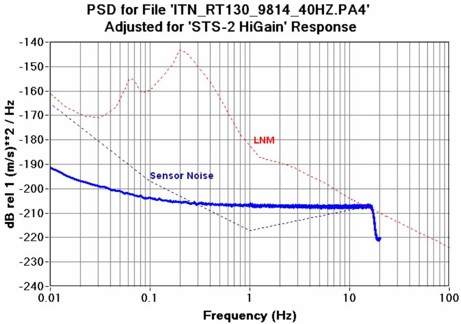
Figure 6.12.6a RT130HR 40SPS CH4 Seismic System Noise STS-2 High Gain
