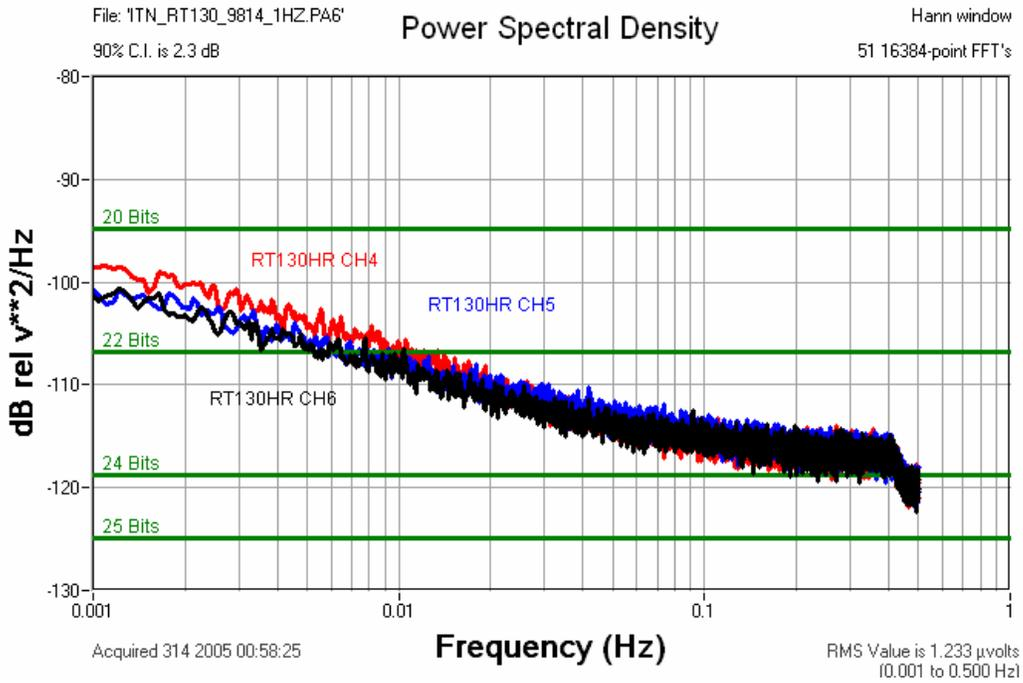
Figure 6.7.8 RT130HR 1SPS Channel 4-6 Input Terminated Noise
