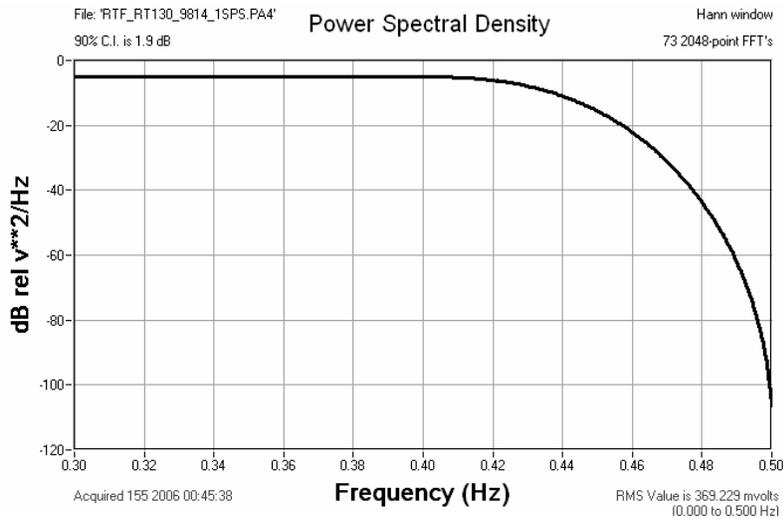
Figure 6.10.5d Response of the RT130HR to Broadband Noise
