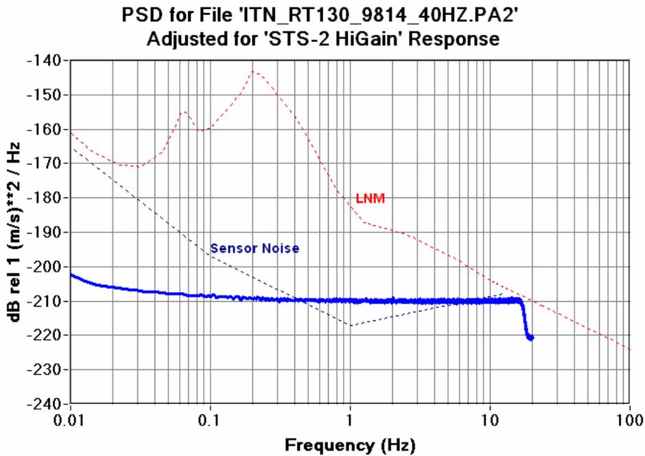
Figure 6.12.4b RT130HR 40SPS CH2 Seismic System Noise STS-2 High Gain
