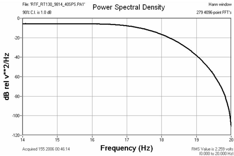
Figure 6.10.3d Response of the RT130HR to Broadband Noise
