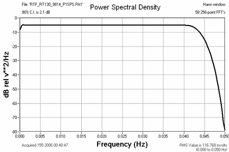
Figure 6.10.6a Response of the RT130HR to Broadband Noise
