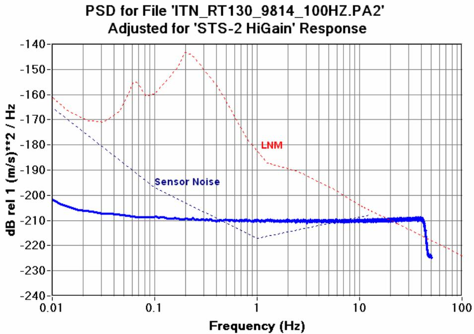
Figure 6.12.2b RT130HR 100SPS CH2 Seismic System Noise STS-2 High Gain
