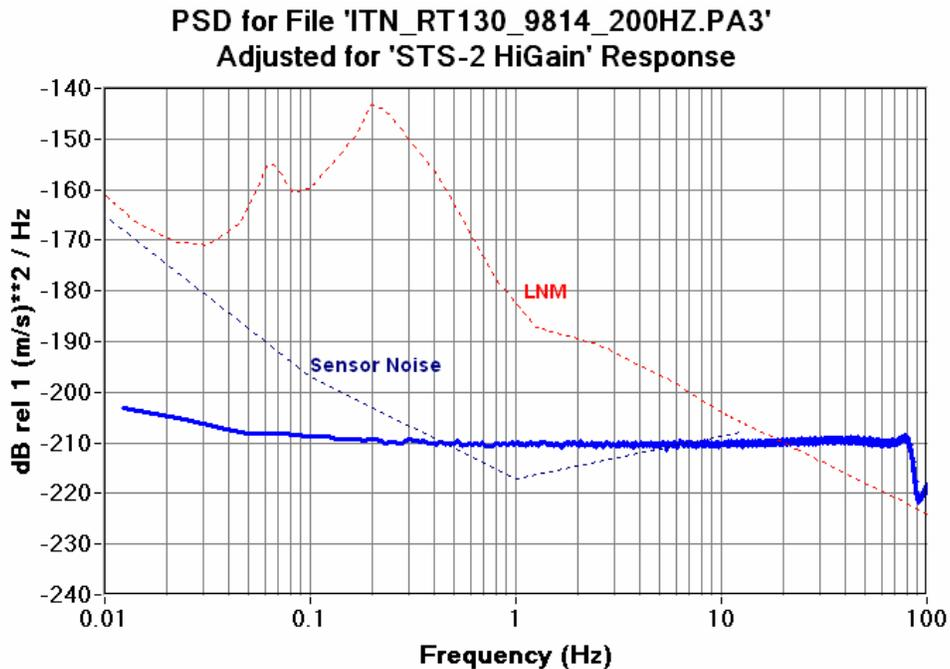
Figure 6.12.1c RT130HR 200SPS CH3 Seismic System Noise STS-2 High Gain
