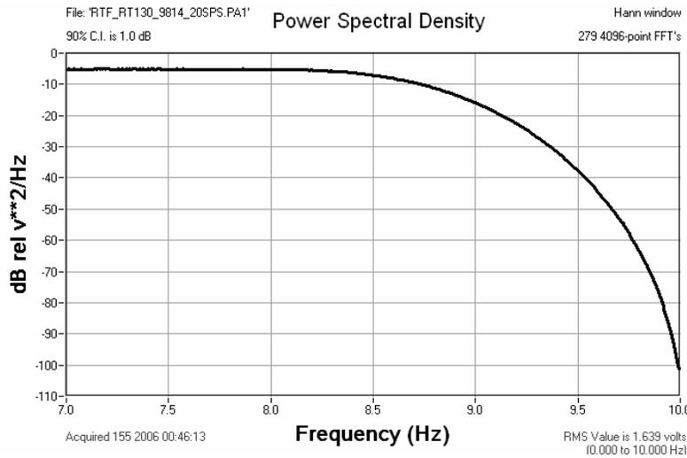
Figure 6.10.4b Response of the RT130HR to Broadband Noise
