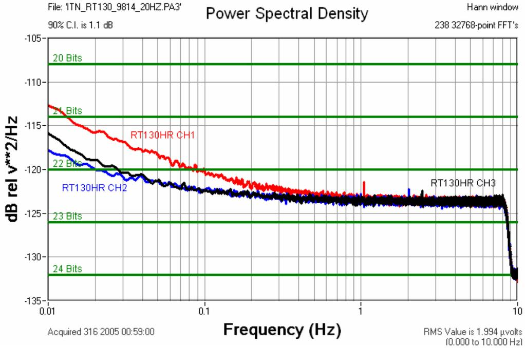
Figure 6.7.6 RT130HR 20SPS Channel 1-3 Input Terminated Noise
