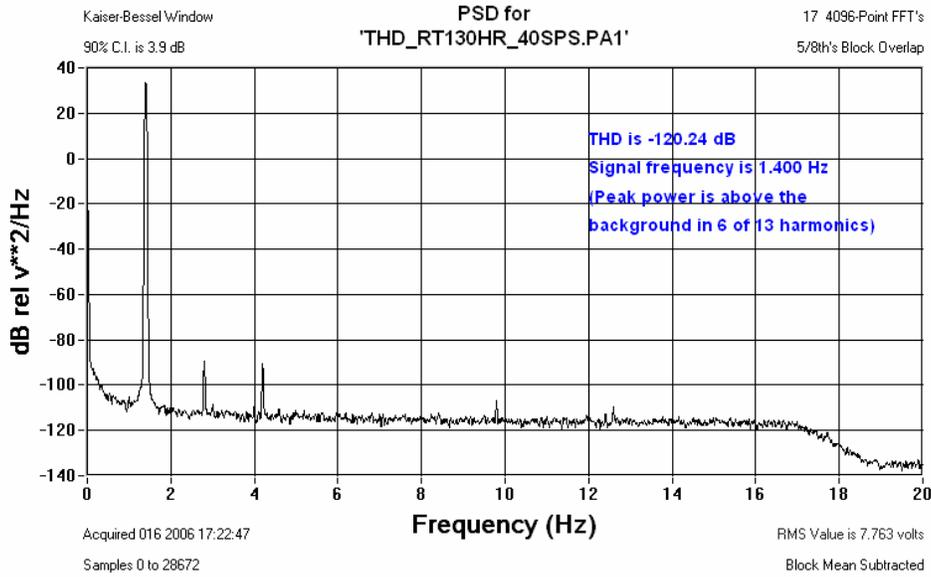
Figure 6.8.1 RT130HR Channel 1 Total Harmonic Distortion
