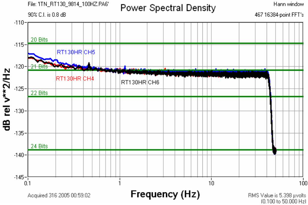
Figure 6.7.3 RT130HR 100SPS Channel 4-6 Input Terminated Noise
