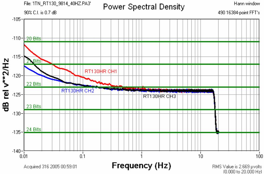
Figure 6.7.4 RT130HR 40SPS Channel 1-3 Input Terminated Noise
