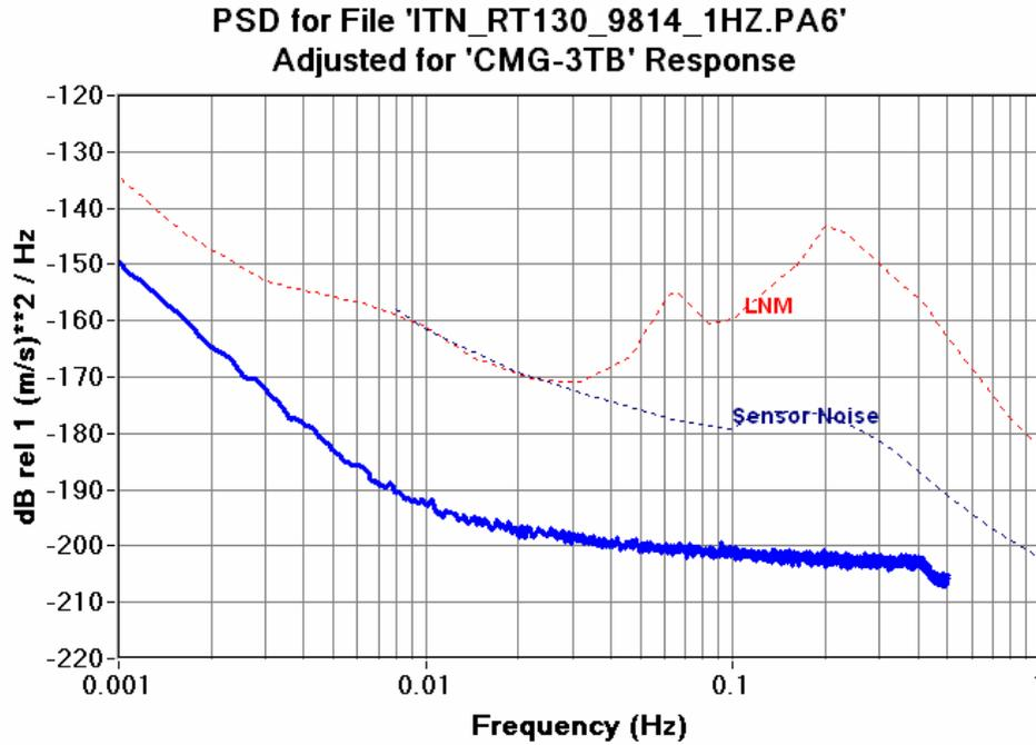
Figure 6.12.15c RT130HR 1SPS CH6 Seismic System Noise CMG-3TB
