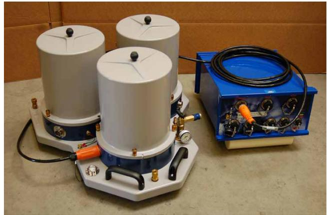
Figure 7.3. Metrozet M2166-VBB triaxial seismometer on the left and M2166-EM electronics module on the right. Metrozet seismometers have been deployed for testing at three GSN stations and ASL to evaluate their potential as a replacement vault instruments. Performance has been documented and subsequent work with Metrozet has resulted in further modifications to improve overall instrument performance.
