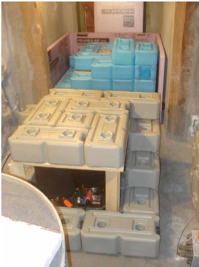
Figure 7.2. Thermal isolation tests on M2166 seismometers at ASL utilize water- or sand-filled containers to dampen the effect of temperature on seismometer noise performance. Preliminary results show considerably slower thermal noise perturbation rates when using water-filled bricks in addition to a standard foam covering.
