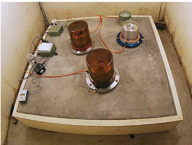
Figure 7.1. The surface vault at IU.CASY (Casey, Antarctica) houses three STS-1 components as well as a STS-2 secondary sensor. This arrangement demonstrates the redundancy built into GSN station design.
