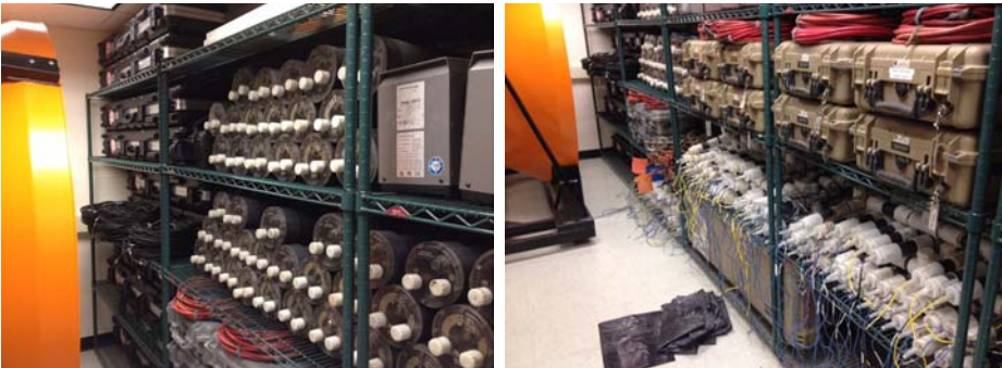
FIGURE MT-1. The current fleet of community magnetotelluric (MT) systems, including three-component magnetometers (left) and receivers and electrodes (right), is sufficiently portable, but aging. New instruments will result in a more robust capacity for portable, PI-led surveys.
