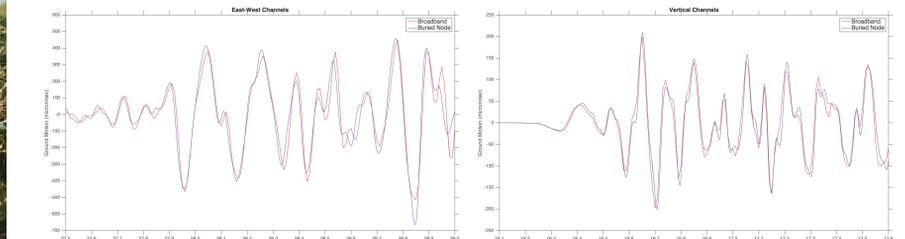
Here we show a comparison between our co-located broadband station (pictured, left) and one of the buried nodes at the same site. These data are from a nearby M4.4 event on 7/9/16 and have been band-pass filtered between 5 and 40 Hz.
