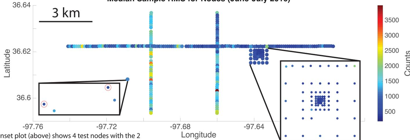
Inset plot (above) shows 4 test nodes with the 2 buried nodes circled in red. Note that the 2 surface nodes (not circled) have higher SAMPLE RMS values.
