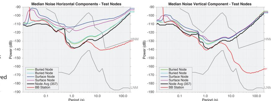
The above spectra show a comparison (horizontal, left; vertical, right) between a co-located broadband, 2 buried nodes, 2 surface nodes, an average spectra for all 357 nodes deployed during the experiment. The nodes deployed are 3-component and have a corner frequency of 5 Hz.
