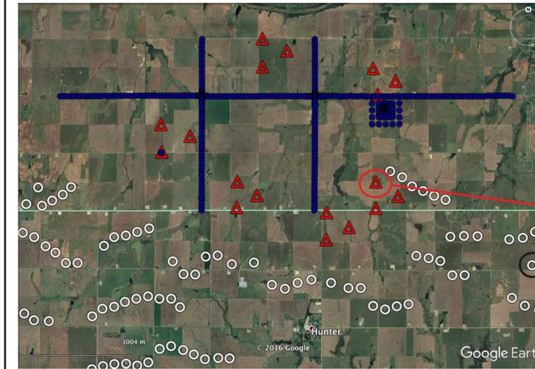
Map of deployment (above) with nodes (blue), broadband stations (red) and wind turbines (white). Below is a plot of local wind speeds and gusts as measured at a nearby airport during the deployment. A calm period (6/28) and windy period (7/12) are shaded and correspond to spectra (right).
