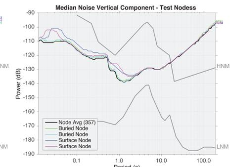
The above spectra show a comparison (horizontal, left; vertical, right) between 2 buried and 2 surface nodes and an average spectra for all 357 nodes deployed during the experiment. The nodes deployed are 3-component and have a corner frequency of 5 Hz.
