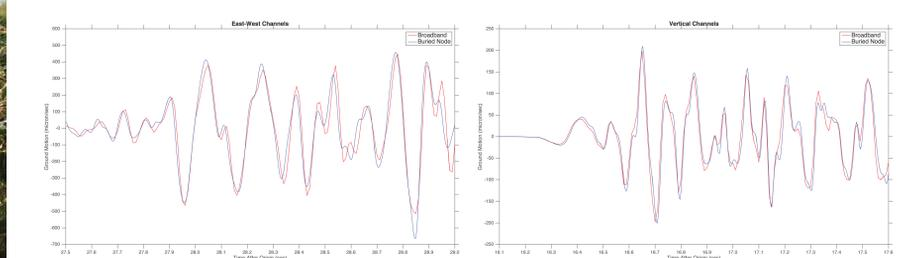
Here we show a comparison between our co-located broadband station (pictured, left) and one of the buried nodes at the same site. These data are from a nearby M4.4 event on 7/9/16 and have been bandpass filtered between 5 and 40 Hz.
