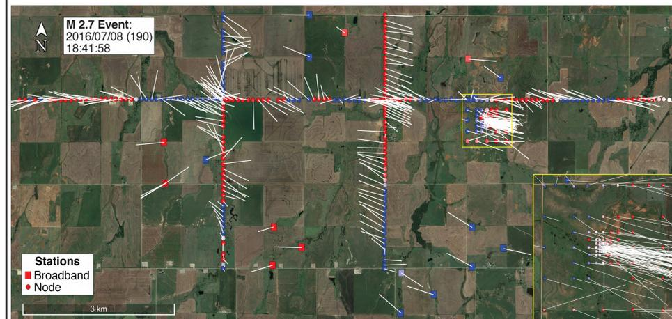
IRIS has produced several ground motion visualizations of the array and we'll show a few of these off using a tablet at the poster presentation. The image above is the array during a nearby M2.7 event (blue=up, red=down, and bars indication horizontal displacement).
