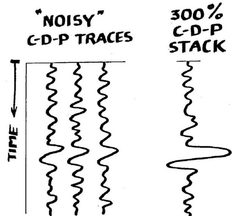
summing 3 traces provides a “stacking fold” of 3
