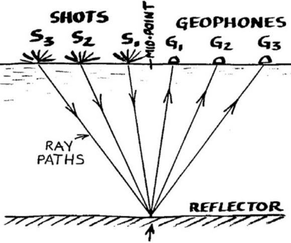
*Trace stacking enhances signal, and reduces noise*
