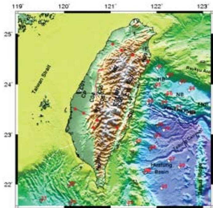
Taiwan and vicinity. The inverted triangles in the offshore area shows the locations of the broadband ocean bottom seismographs. Currently 20 of them are being occupied. The inverted triangles on land marked the site of TAIGER stations from PASSCAL.
