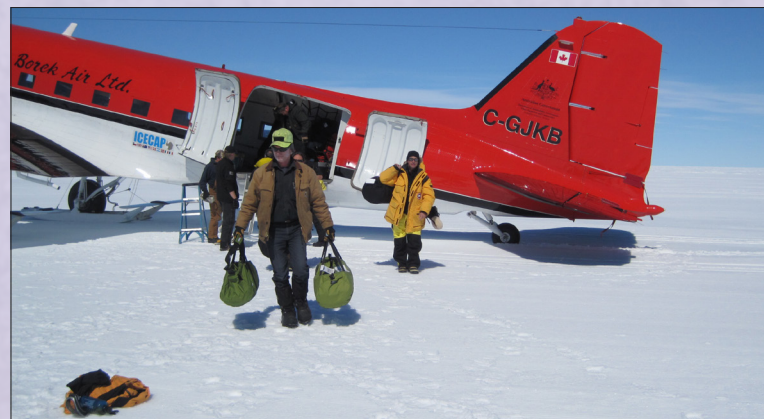
Field engineers from ASL arrive at CASY (Casey Station, Antarctica) to perform an upgrade the GSN station. Travel is via an updated DC-3 on skis called a Basler.
