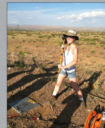
Intern Rachel Petit takes her turn using the hammer seismograph during the 2012 intern orientation at New Mexico Tech.
