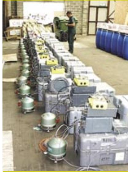
new Texans have four times as much memory, allowing higher sample rates, longer recording times, and more shots per deployment. Yet they can be redeployed more quickly than the old Texans thanks to an even greater increase in data upload speed. New data loggers for passive experiments introduced during 2004 have proven more reliable than the older units, in addition to being lighter and providing IP connectivity. Experiment support has been enhanced through development of
