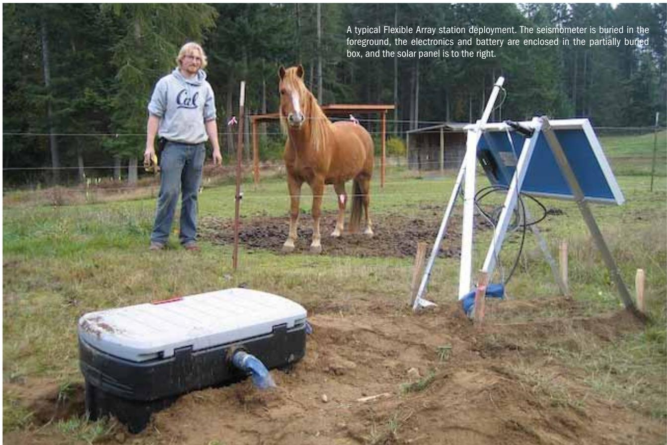
A typical Flexible Array station deployment. The seismometer is buried in the foreground, the electronics and battery are enclosed in the partially buried box, and the solar panel is to the right.
