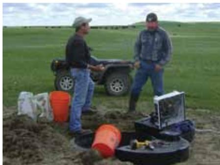
Scientists align a magnetometer in the vault of a permanent Magnetotelluric station.
