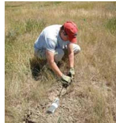
University of Colorado PI Anne Sheehan buries a Texan geophone for the Bighorn Arch Seismic Experiment (BASE). The data logger is bagged and also buried to reduce temperature fluctuations inside the unit. This seismometer is powered by two D-cell batteries. (Photo: Anne Sheehan)
