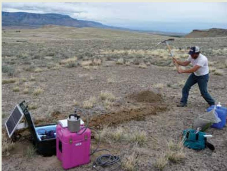
Jeremy Silver (CU) digging a trench for the short period seismometer's cables. The seismometer, in the pink box, will be buried at the end of the trench. The battery, GPS, and data logger are in the box with the solar panel and will be left on the ground all summer. (Photo: Anne Sheehan)
