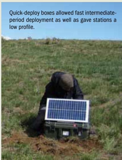
Quick-deploy boxes allowed fast intermediate-period deployment as well as gave stations a low profile.
