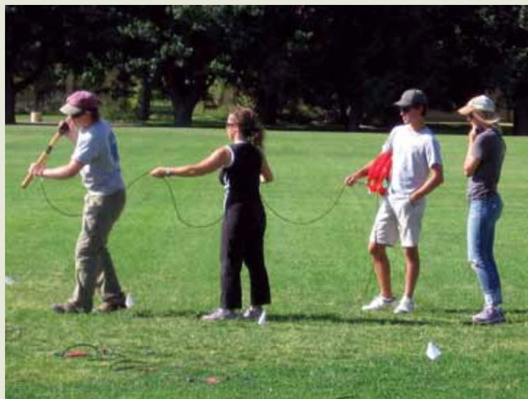
Using a hammer seismograph at the Intern orientation.
