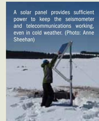
A solar panel provides sufficient power to keep the seismometer and telecommunications working, even in cold weather. (Photo: Anne Sheehan)
