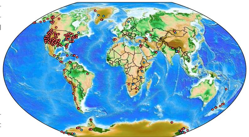
Locations of active experiments using IRIS portable seismic instrumentation from January 2015 through December 2019. Blue dots (49) denote experiments started prior to January 2015 but that were still active during the timeframe. Red dots (271) are experiments initiated after January 2015.
