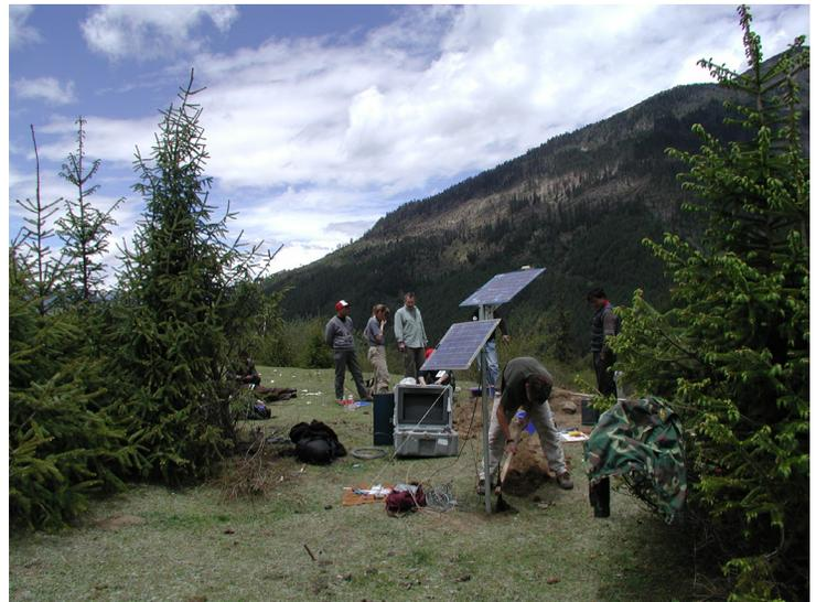
Designed as small, light weight, and easily deployed instruments, the single-channel DAS are primarily used for active source reflection and refraction surveys. Once deployed, the units can run for 7 to 10 days on a single pair of "D" cell batteries. Data are stored in internal flash ram, ranging in size from 32 Mbytes to 256 Mbytes, at sample rates up to 1000 sps. An internal oscillator is synchronized to GPS time before and after deployment.
