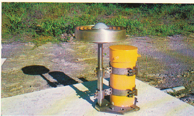
Picture: GPS antenna mount and benchmark coupled to the seismometer casing wellhead at MSEY (Mahe Island, Seychelles; photo by Garth Franklin, JPL).
