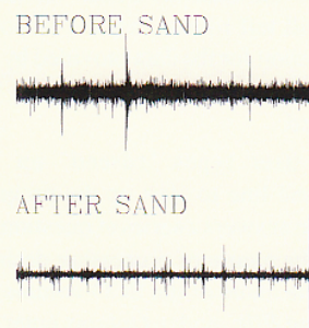
Figure 2. Seven day time domain records in the 20 to 600 second pass band of relative noise levels in sand and no-sand installations.
