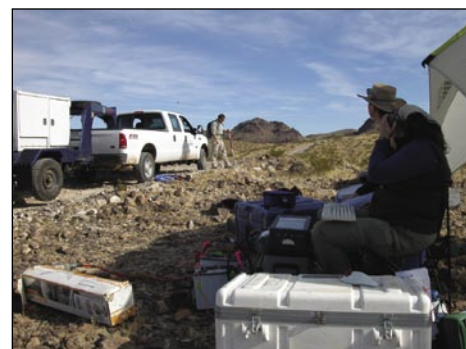
Our most recent high-resolution seismic reflection survey in the River Mountains using our mini-vibe source.
