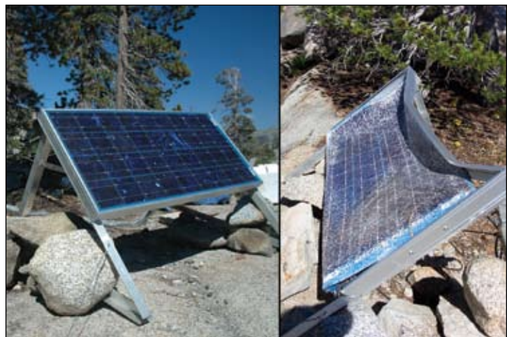
Solar panel at SNEP 75 (northwestern edge of Yosemite National Park) before (left) and after (right) a winter with probably more than 8.5m peak snow depth.
