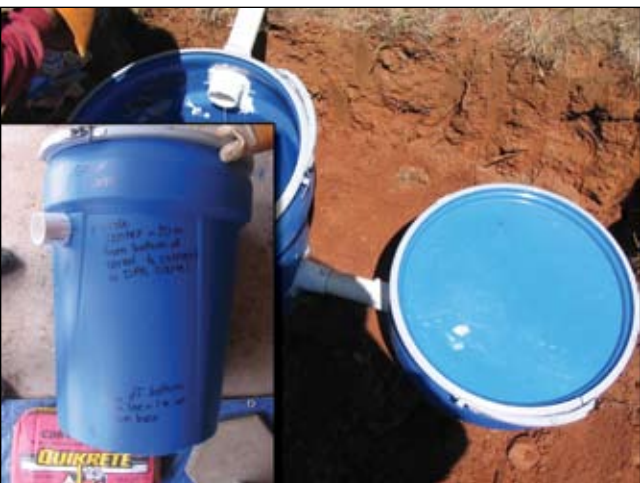
New vault design for SNEP phase 2 uses airtight top with open bottom for both sensor and electronics.
