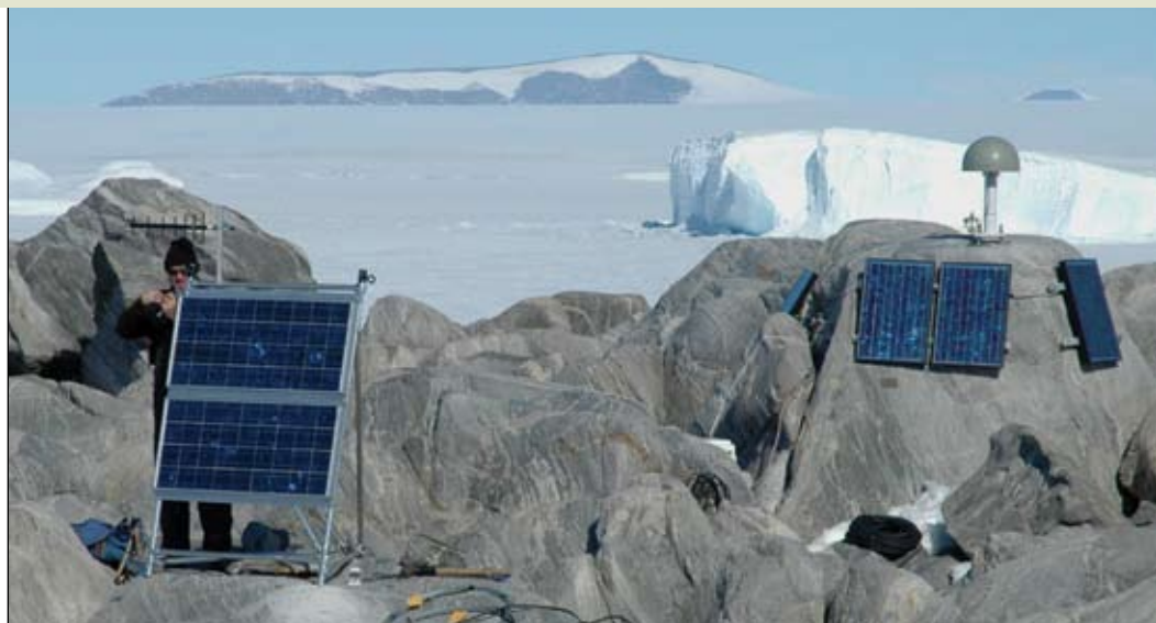
Seth White upgrading the power system at the Cape Roberts continuous GPS site.
