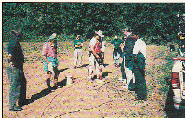
Bill Stephenson of the U.S.G.S. demonstrates the use of a shotgun source in Shallow Seismic Profiling.
