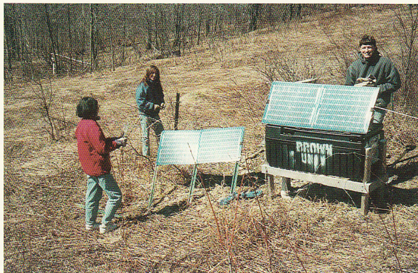
Figure 2. View of MM04 (LeRaysville, PA). The black box contained the DAS, SCSI disk, and two marine batteries. The sensor was located in a buried vault roughly 8' behind the solar panels. The photo also shows Brown University students Matthew Fouch, Julie Zaslow and Aibing Li (right to left) in the process of demobilizing the station. MM04 was located in a field behind the LeRaysville Cheese Factory which made it a very popular stop on array maintenance trips.
