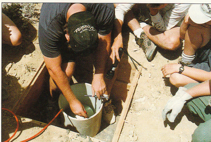
Photo 2. Training session for installation of the STS-2 seismometer in an IGPP "mini-vault". The mini-vault has been oriented to true North by gyrocompass and set in quick drying cement. The field technician is leveling the seismometer before installing the waterproof lid and insulation.
