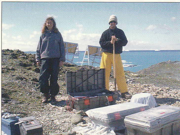
Figure 2. Washington University graduate student Stacey Robertson and Universidad de Chile graduate student Kenneth Lein finish installing the unattended broadband station at Low Island in the Antarctic. During the summer, the station is powered by arrays of solar panels (background), whereas during the winter, power is provided by 18 Carbonaire batteries, located in the plastic bins (foreground).
