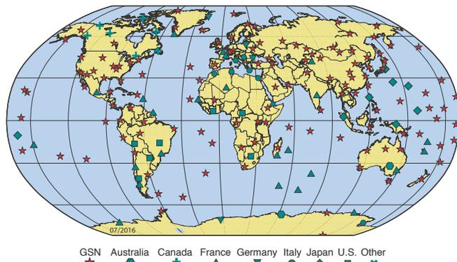
**FIGURE GSN-1.** Distribution of GSN stations (red stars) and the International Federation of Digital Seismograph Networks (FDSN) backbone stations (green symbols). The GSN avoids duplication of coverage by taking into account the locations of quality FDSN stations. The GSN is jointly operated by IRIS, with funding from the NSF, and the USGS's Albuquerque Seismological Laboratory.
