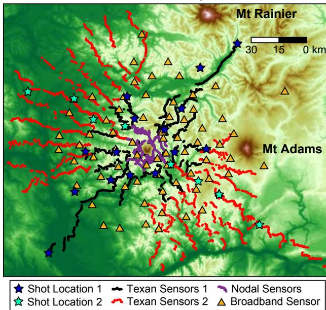
**FIGURE ISF1-1.** The deployment of nodal instruments across the top of Mount St. Helens for the iMUSH experiment is an excellent demonstration of using dense sensor spacing in a challenging environment. This experiment used nearly 6000 seismic sensors, including 70 broadband seismographs, 4981 geophones with “Texan” recorders deployed in two phases, and 920 nodal sensors.
