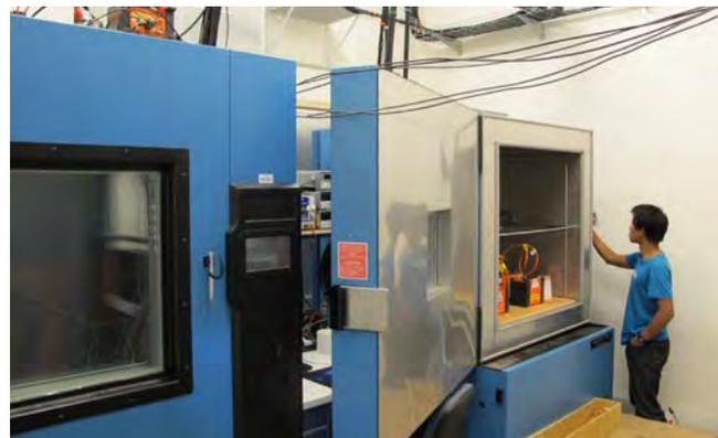
**FIGURE PL-3.** Cold chambers in a specialized room at the PASSCAL Instrument Center allow testing of components and systems in expected field environmental conditions.
