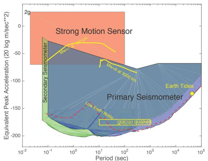
**FIGURE GSN-2.** The GSN deploys multiple sensors at each station to achieve the design goal of recording many types of signals on scale and with full fidelity. No single sensor can capture all data of interest.
