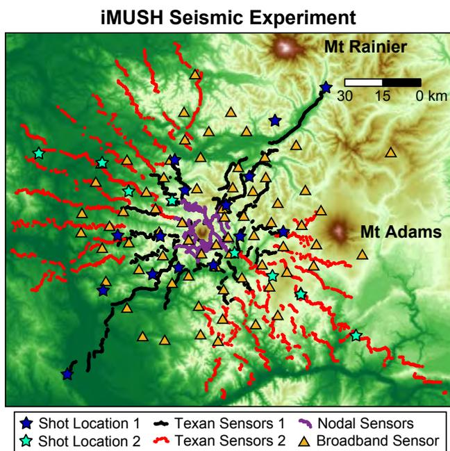
**FIGURE ISF1-1.** The deployment of nodal instruments across the top of Mount St. Helens for the iMUSH experiment is an excellent demonstration of using dense sensor spacing in a challenging environment. This experiment used nearly 6000 seismic sensors, including 70 broadband seismographs, 4981 geophones with “Texan” recorders deployed in two phases, and 920 nodal sensors.
