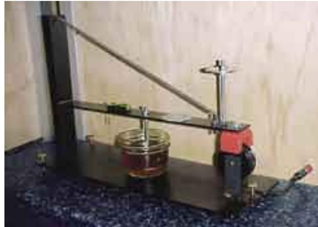
The AS-1 is an affordable seismometer that is robust enough to be operated in high schools and that transparently demonstrates seismometry principles.
