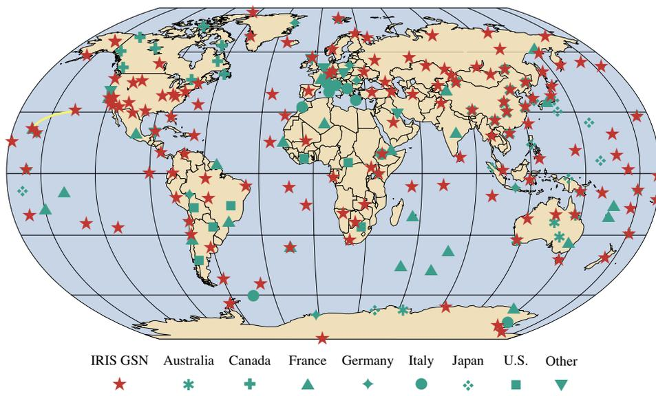
Distribution of stations in the Federation of Digital Broad-Band Seismograph Networks, highlighting the major contribution of GSN to the global coverage, complemented by that of its national and international partners, and a significant number of stations installed and operated jointly by GSN and various FDSN partners.
