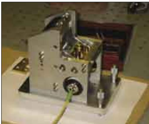
Figure 2. Prototype Vertical Optical Seismometer. This unit has a mass of 360 grams and a free period of a few seconds. The spring is a single strip of "NiSpan-C", a trade name for a particular alloy of iron-nickel with small amounts of chromium and titanium.
