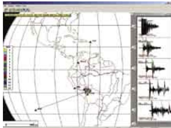
**EqSelect:** Allows the student to select P-arrivals and use these to locate an earthquake iteratively. Seismograms can be downloaded from the IRIS Wilbur site or from schools which share their seismograms.
