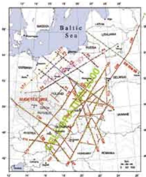
Figure 2. Index map showing the locations of major seismic refraction experiments in Central Europe.
