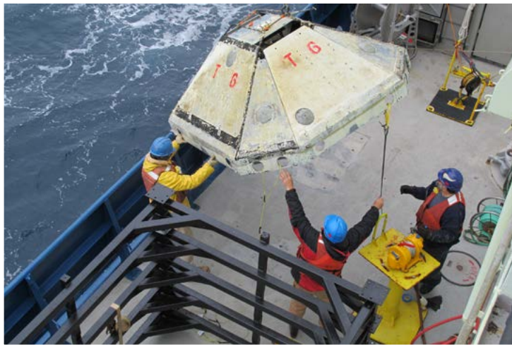
Figure 36. Repositioning an LDEO TRM as it is recovered aboard R/V Atlantis. Photo credit: Cruise AT26-02
