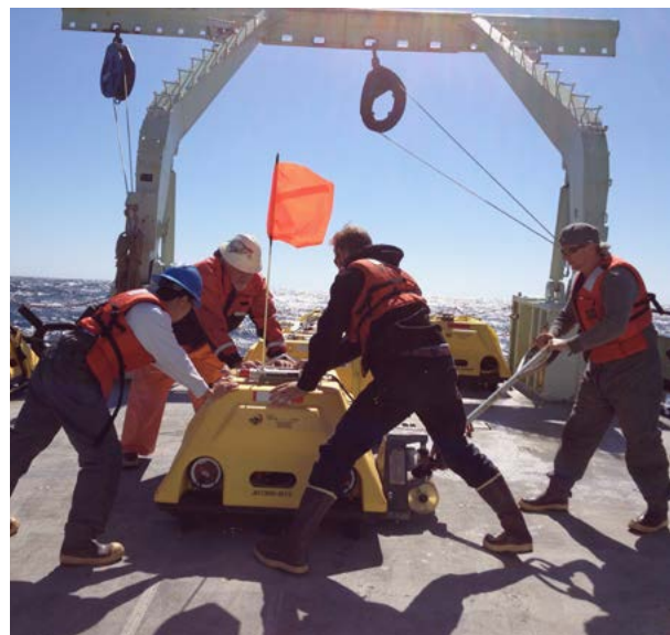
Figure 1. A Scripps Institution of Oceanography (SIO) Abalone OBS is moved into position for deployment aboard R/V Oceanus by SIO OBS crew Phil Thai and Martin Rapa, Marine Tech Erik Arnesen, and Bos'n Doug Beck. Photo credit: Cruise OC1208B
