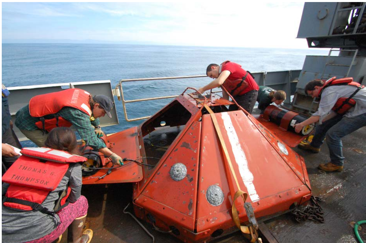
Figure 5. Two watches converge to quickly deconstruct a trawl-resistant OBS. From left to right: Melodie Elmer, Nick Benz, Sam Bell, Rose Wade, and Blake Parris. Photo credit: Erik Fredrickson
