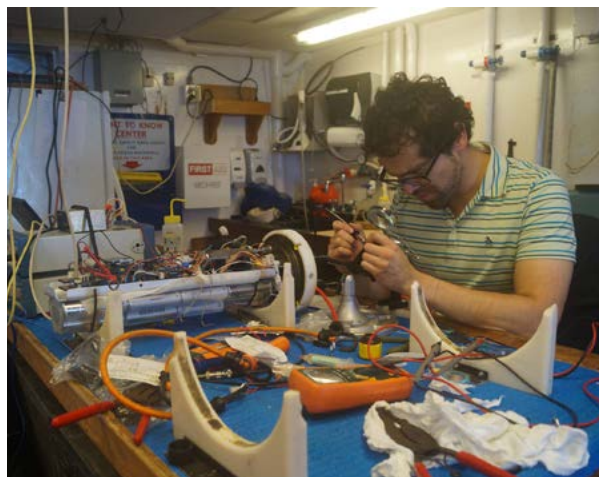
Figure 14. LDEO Engineer Carlos Becerril modifies an instrument's circuits before it is deployed at sea aboard R/V Oceanus . Photo credit: Cascadia Initiative Expedition Team
