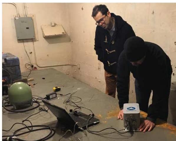
Figure 9. LDEO Engineer Carlos Becerril and ASL Engineer Jared Anderson mark new north lines on the LDEO instrument testing pier using an Octans. Photo credit: Kasey Aderhold
