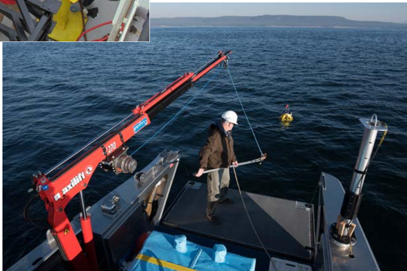
Figure 37. WHOI engineer Tim Kane stands ready to hook and recover an OBS from Yellowstone Lake. In compliance with the research permit, the anchor needed to be recovered as well as the instrument. Photo credit: Chris Linder, Woods Hole Oceanographic Institution
