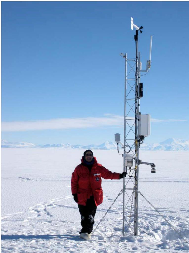
FIGURE 5: A new University of Wisconsin-Madison Automatic Weather Station (AWS), located at Elaine Site on the Ross Ice Shelf, Antarctica, measures temperature at two levels, atmospheric pressure, relative humidity, relative snow accumulation, solar radiation, wind speed and direction. The AWS systems have provided reliable meteorological data on very low power budgets and infrequent servicing visits.
