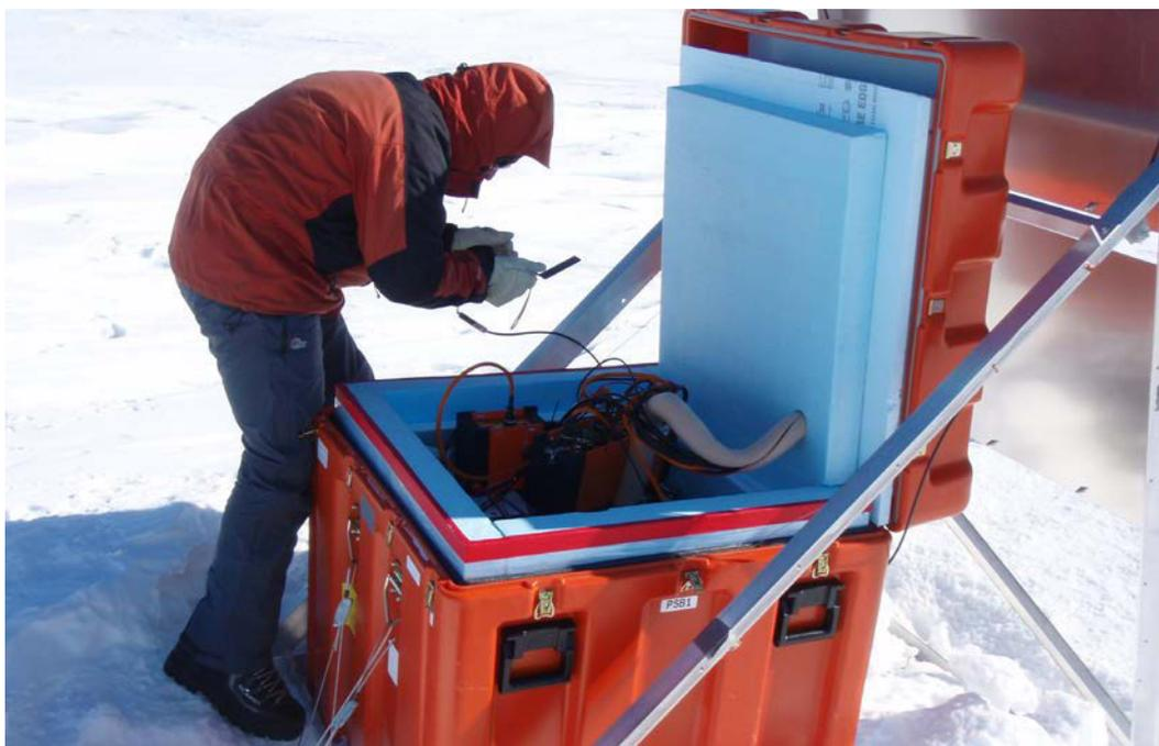
FIGURE 1: Andrew Lloyd, a Penn State graduate student, servicing an Antarctic seismograph site for the POLENET/ANET project. Operating instrumentation in polar regions poses numerous logistical and environmental challenges for both equipment and personnel.
