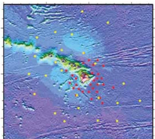
**Figure 9.** Distribution of broadband ocean bottom seismometers in the PLUME experiment around Hawaii. Red: first deployment. Yellow: second deployment. Blue: island stations.
