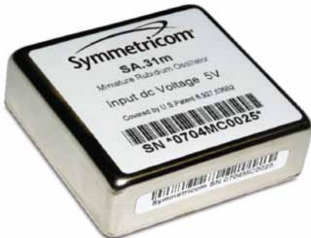
**Figure 21.** A photo of the Symmetricom SA.31m atomic clock on a chip. The dimensions are 51 mm x 51 mm x 18 mm (high). Approximately nine minutes are required to heat the oven to control temperature during which time the clock draws 14 W. The clock's accuracy, when on as an atomic clock, is  $< 7 \times 10^{-10}$ . The clock will operate only occasionally to discipline the TCXO.
