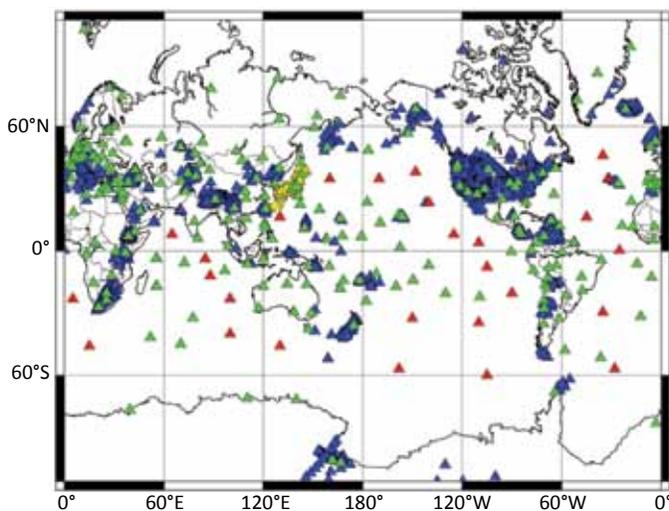
**Figure 8.** Distribution of seismic stations. Red triangles: possible locations of ocean bottom instruments to fill in gaps left by land stations. Green and yellow: Global Seismographic Network, Japan network, and other permanent stations. Blue and black: deployments of broadband instruments in array experiments. From S. Tanaka presentation, EPOBS workshop.
