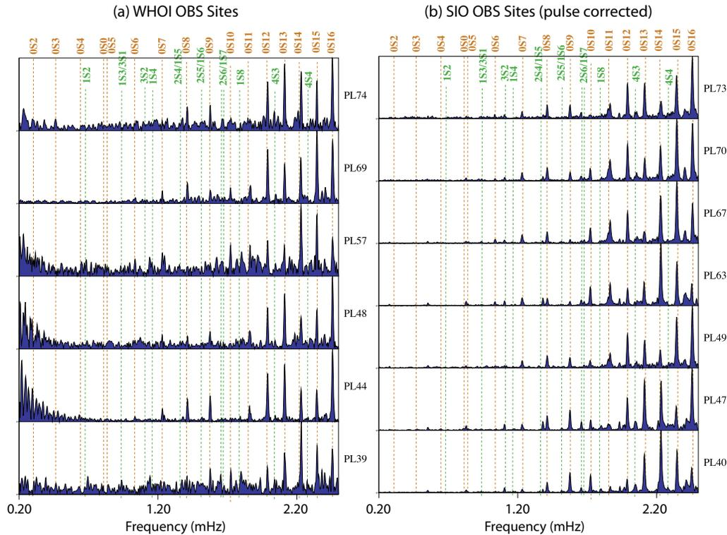
**Figure 19.** Vertical component spectra for the Kuril event from data recorded for 50 hours beginning 1.5 hours after the event time. (a) plots the best six CMG-3T sites while (b) plots seven of the eight Trillium seismometers. Figure courtesy of G. Laske.
