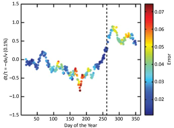
**Figure 7.** Changes in velocity of 1 s period Rayleigh waves associated with an  $M_w$  6.0 earthquake on the Gofar transform fault (McGuire et al., 2012). Vertical dashed line indicates time of earthquake. Velocity or travel time is measured using ambient noise correlation between two sites on the fault. Note that the change in velocity or travel time appears to begin before the earthquake, suggesting it may be possible to make a short-term forecast of an impending event.
