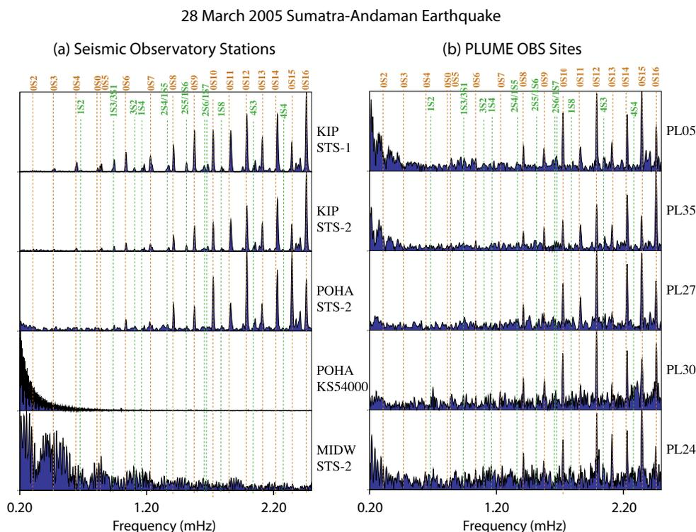
**Figure 18.** Vertical component spectra for the Sumatra-Adaman event using 50 hr segments beginning 90 min after the event. Modes are clear on both the STS1 and STS2 at KIP (Oahu) while at POHA (Maui), the only operating sensor (STS2) recorded free oscillations. These were not recorded at an STS2 at Midway. Five of the best WHOI CMG-3T OBS power spectra are depicted in (b). The Trillium 240s were not deployed in the first annual window of the experiment. Figure courtesy of G. Laske.
