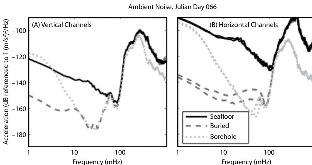
**Figure 12.** Noise-level comparison of seafloor, borehole, and shallow-buried seismometers from an experiment south of Hawaii. Figure courtesy of J. Collins.
