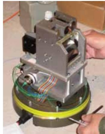
**Figure 23.** A modified Streckeisen STS1 seismometer, termed an iSTS1, has no electrical connections and no feedback for mass centering.
