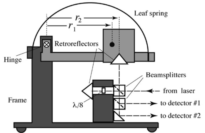
**Figure 22.** Illustration of the use of two laser beam splitters and a retroreflector on the mass to provide two beams to an interferometer, which measures the phase difference generated by the mass' position.
