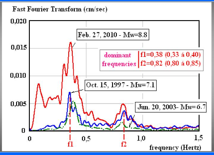
FAST FOURIER TRANSFORM OF THREE OF THE CHILEAN ACCELEROGRAMS RECORDED IN LA PLATA
