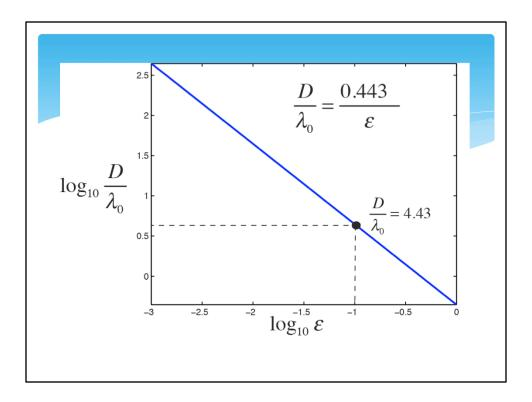
This is a plot of of the needed array diameter to target wavelength ratio for different desired error thresholds. Smaller separations in slowness require greater array diameters.
