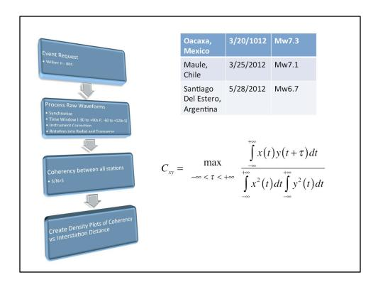
The data were processed in this manner. The maximum of the normalized correlation coefficient gives an estimate of waveform coherency of two waveforms. The coherency estimate is plotted with respect to interstation distance as the proxy for wavelength.
