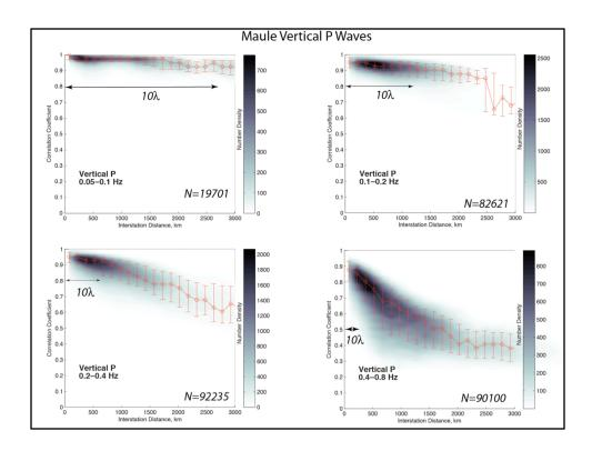
Here are the results for Maule P waves for 4 different bandpasses. The number density of coherency is plotted versus interstation distance. "N" is the number of coherency estimates. Note that P waves are highly correlated to distances greater than 10 wavelengths. The "error bars" show the width of the number density peak at half value.
