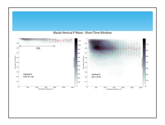
Using a short time window inversely proportional to the bandpass center frequency necessarily increases the wave coherency. Here, even 1.2Hz P waves appear highly correlated across USArray (although there is large spread).
