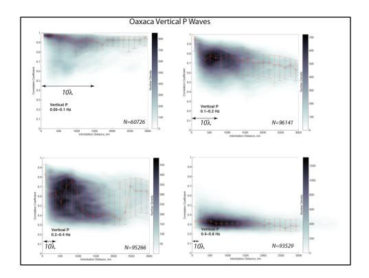
Correlations for Oaxaca P waves for the fixed time window. There is a large spread in the correlation density although peak values at low frequency are generally highly correlated. Decorrelation of most bandpasses may reflect the effect of upper mantle structure, e.g., P wave triplications.
