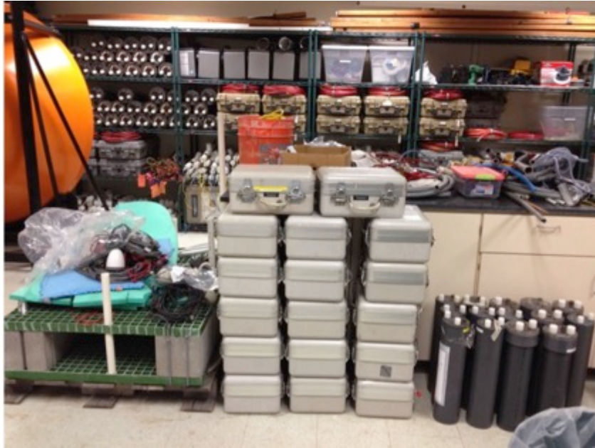
Caption: A view of part of the current inventory of the National Geoelectromagnetic Facility's land EM instruments (EM receivers, magnetic field sensors, electric field sensors)
