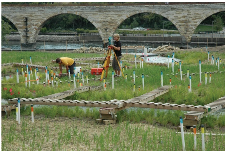
Figure 2.21 The Outdoor StreamLab (OSL) facility at the National Center for Earth Surface Dynamics (NCED), located on the banks of the Mississippi River at the University of Minnesota, is dedicated to stream restoration research. OSL uses an abandoned flood bypass channel near St. Anthony Falls to study interactions among river channels, floodplains, and vegetation. Dams and bridge piers can be added to the OSL channel to investigate human-river interactions. SOURCE: Available at www.nced.umn.edu/content/outdoor-streamlab-osl . Courtesy of the University of Minnesota.
