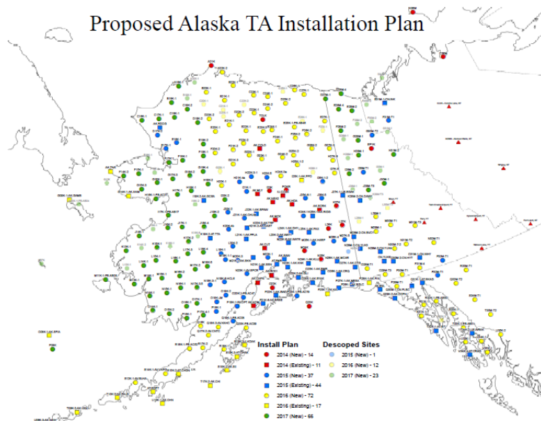
Figure 1 Planned stations of the Alaska Transportable Array. Red symbols are currently operating, Blue are being installed this summer, while Yellow and Green are planned for FY16 and FY17. A total of 261 stations are planned for operation up to 2019 or beyond.
