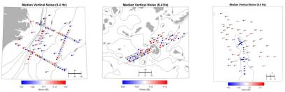
The maps above display the median PSD for each station, at a frequency of 6.4 Hz, over the entire recording period. Spatial differences in performance are revealed, such as higher noise in shallower waters. At 6.4 Hz the stations in Lake Malawi perform much better relative to the land stations deployed as part of this experiment.
