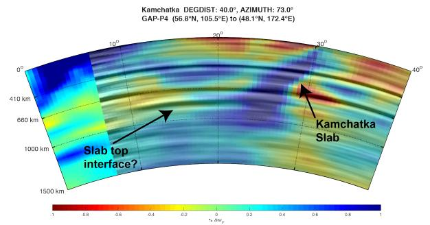
Apparent reflectors/discontinuities from stacked *SS* precursors superimposed on the GAP\_P4 *P*-wave tomography model [*Obayashi et al.*, 2013] along a cross section of the Kamchatka slab. Dark stripes represent strong reflectors and discontinuities across which *S*-wave impedance increases dramatically.
