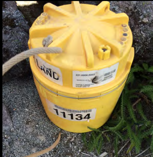
Geophone response peak at 10 Hz
