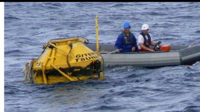
Figure 18. German GITEWS Tsunami Buoy – Stolen Superstructure and Buoy Payload
