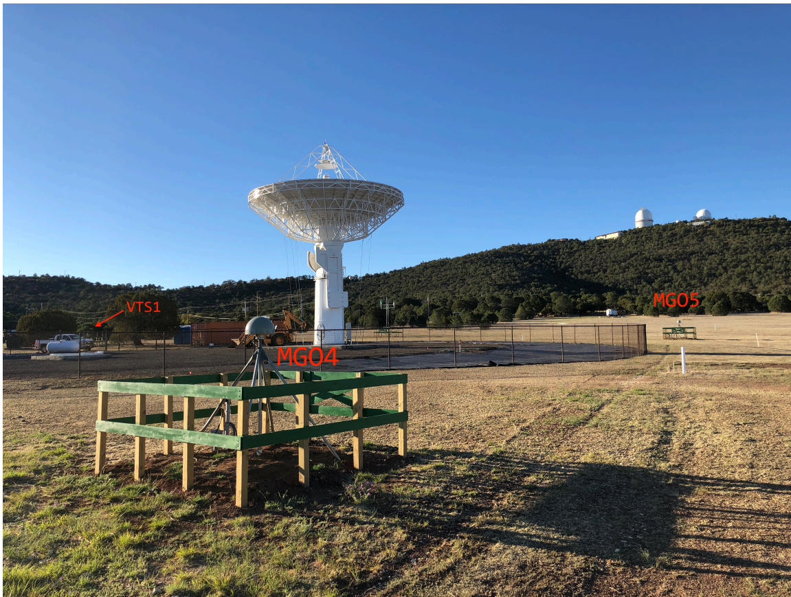
Image – The SGP VLBI instrument at the McDonald Observatory near Fort Davis, TX, surrounded by three UNAVCO-installed GNSS stations. Optical astronomical telescopes are visible on the hill in the background. (Photo credit: J. Sklar, UNAVCO)
