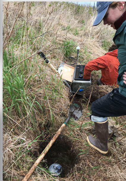
Direct-burying direct-bury sensors is fast and reliable
