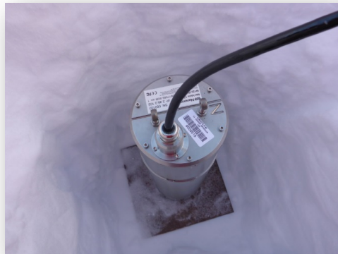
Direct-burying direct-bury sensors is fast and reliable
