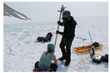
Kristin Poinar and Erasmus Oware of the University at Buffalo deploying a seismoelectric test at Taku Glacier, Juneau Icefield, Alaska in 2019. The seismic source (akin to a Buffalo gun or a Betsy gun) detonates  $\sim 1.5$  meters below the surface of the ice and sounds the englacial environment to hundreds of meters depth.
